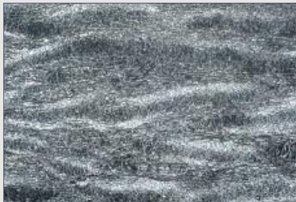
Cellulose acetobutyrate top coat with plasticiser - no defects marked
