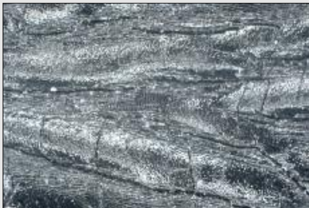
Nitrocellulose top coat without plasticiser - some defects marked
