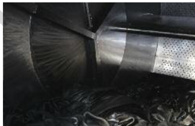
Examples showing deep shelf drums being used for dye/retan/fatliquor. The leading edge of the shelf can be profiled, and different drainage arrangements enable recirculation of floats.
