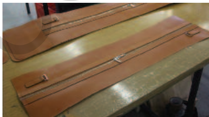
Zip parts ready for fitting to travel bag. CREDIT: WTP
