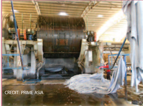
Wet back drums at PrimeAsia's tannery in Vietnam make ensures that water is used more than once.
