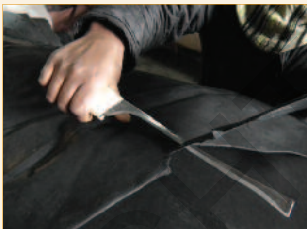
All of the knives used for trimming throughout the tannery are made from used splitting blades.
