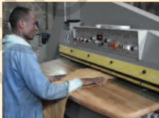
For accuracy of substance, bovine leathers are often dry shaved. These leathers – black and selected colours – often demand very intense colour, and in this event are re-dyed.
