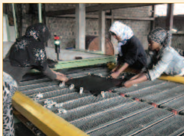
These leathers are being dried on a horizontal throughfeed toggling unit after staking and dry milling.
