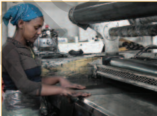
The finishing department is fitted with two finishing lines comprising a single roller-coating machine and a spraying unit.
