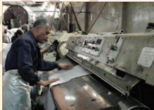
Sheepskins and bovine hides are processed using the same drums and in the same wet processing department, but this shaving machine is dedicated to shaving bovine wet blue.
