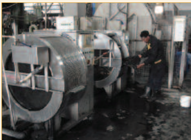
The pilot plant comprises both stainless steel and wooden drums of various sizes for development work and sampling purposes.
