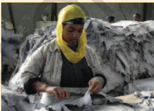
After shaving, sheepskins, bovine sides and bovine splits are trimmed in one area in preparation for dyeing and retanning in a single bank of dyeing drums.
