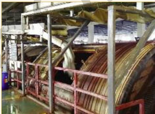
Shows the delivery of a lime split hide from the overhead conveyor delivery system into the selected tanning drum.
