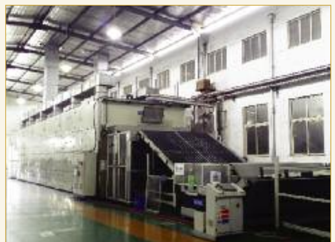
After vacuum drying, hides are manually transferred to a conveyor feeding a wet stretching/staking machine, followed by TAIC drying.
