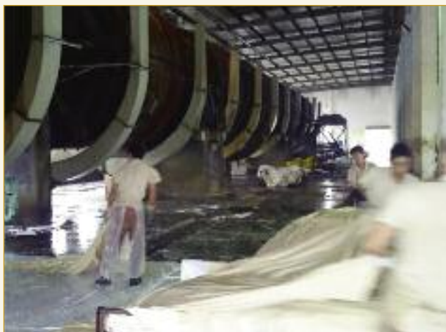
After tanning, hides are stacked down flat on pallets for 24 hours to improve fixation of the tanning agents.
