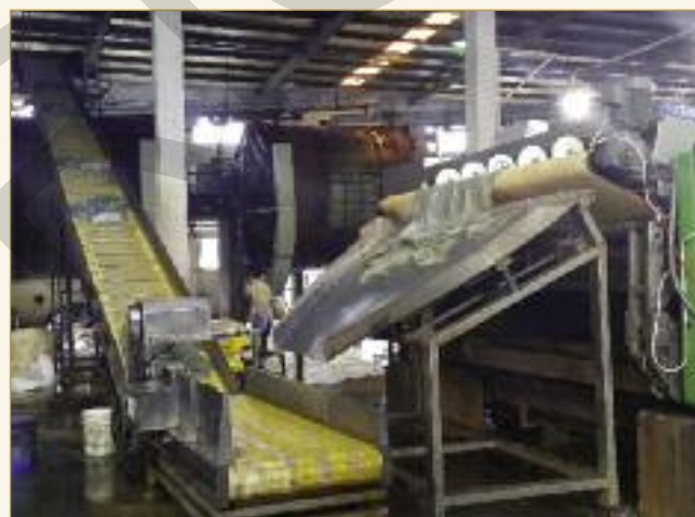
After lime splitting, the grain split from each hide drops onto a conveyor for delivery to the designated tanning drum.
