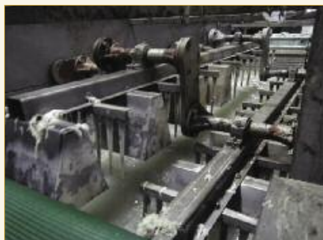
After spraying on the flesh side with sodium sulfide to loosen the wool, the skins are mechanically pulled to remove the wool from the skin. This is of high value, and is immediately machine-washed as shown above to clean and ensure the complete removal of residual sulfide before scouring.
