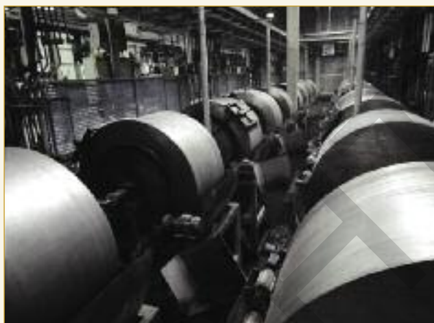
The dyeing department is highly automated with both the additions of skins to process, and additions of water and chemicals under computer control. There are both wooden drums by Olcina, and stainless steel vessels as shown by Capdevila.
