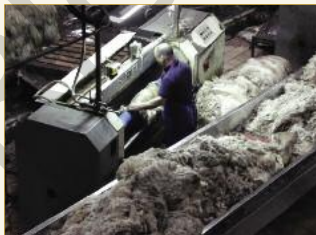
Belt transport of sheepskins after soaking for presentation to the fleshing operation. This stage is especially important to ensure both a clean flesh and remove grease. These sheepskins are for nappa leather production and wool recovery.
