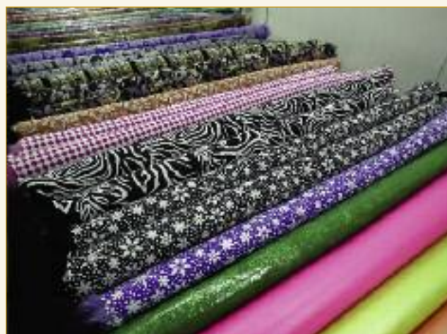
Double-faced sheepskin leathers were traditionally produced as suede with wool of varying length to suit purpose. This variety of finishes is created by laser printing and transfer systems for use mainly in footwear.
