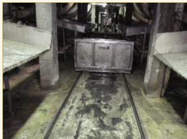
After liming and deliming, the skins are dropped from the paddle via chutes into a Caravel unit. This will automatically transport the load on rails towards a conveyor belt, then tip the skins onto the conveyor belt for delivery as required to wet back or pickle fleshing.
