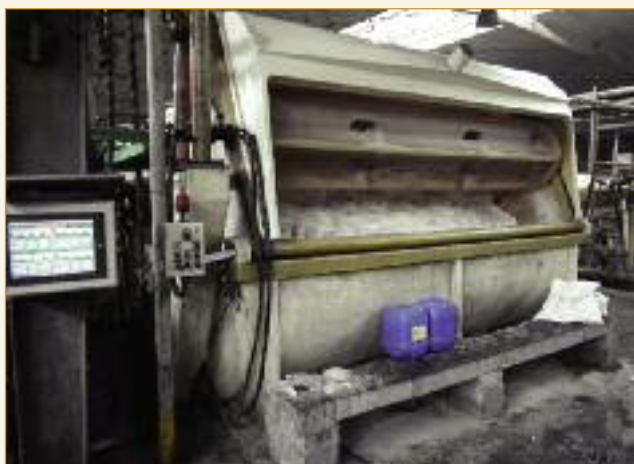
Paddles of 5000 litre capacity are constructed with an inner perforated shell that enables the load to be rapidly drained, then raised and tilted to assist unloading. The floats can be separated on discharge from each paddle for screening, making up to strength and recycling. The system includes computer management.
