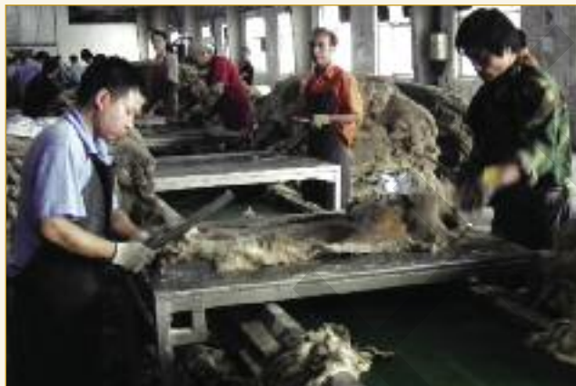
There are 20 tables used for trimming the salted sheepskins, and all are served by a central conveyor for removing the offcuts. The trimming knives are made from used band-knife blades.
