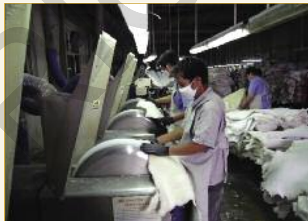
The double-faced sheepskins are dry wheeled after toggle drying and before dyeing.
