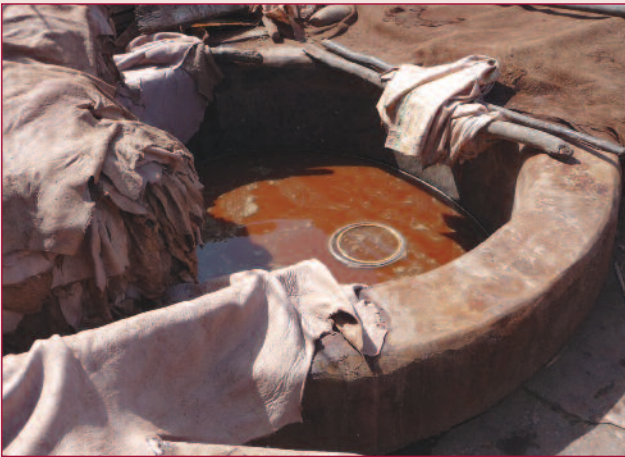
The next stage is a 20-day tanning period. Various natural tanning materials are used to provide colour, and the pits are covered to avoid bleaching by sunlight.
