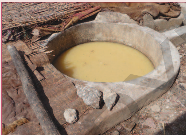
Goat skins are soaked in lime solution only for 10-days. They are hauled out daily and re-immersed in the solution.
