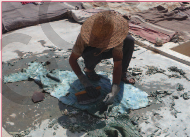
The alkali swollen flesh is then removed from the skins using a shaped flat bladed tool.
