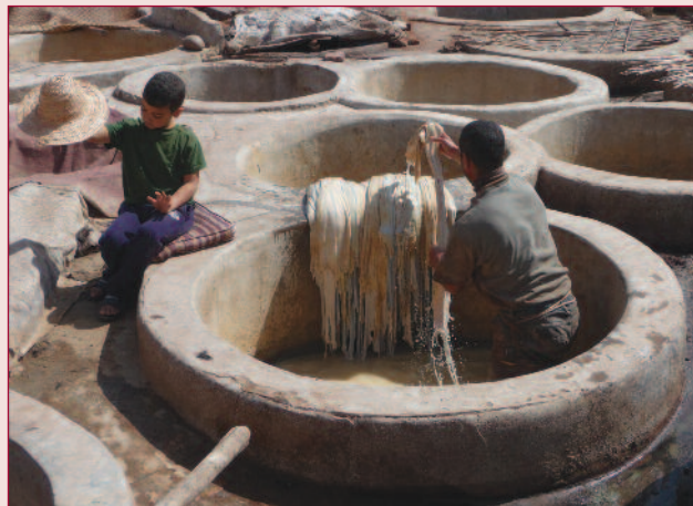
To neutralise the alkalinity, deswell and soften the skins they are immersed in a solution of pigeon dung. They are turned regularly as shown over a 15-day period.
