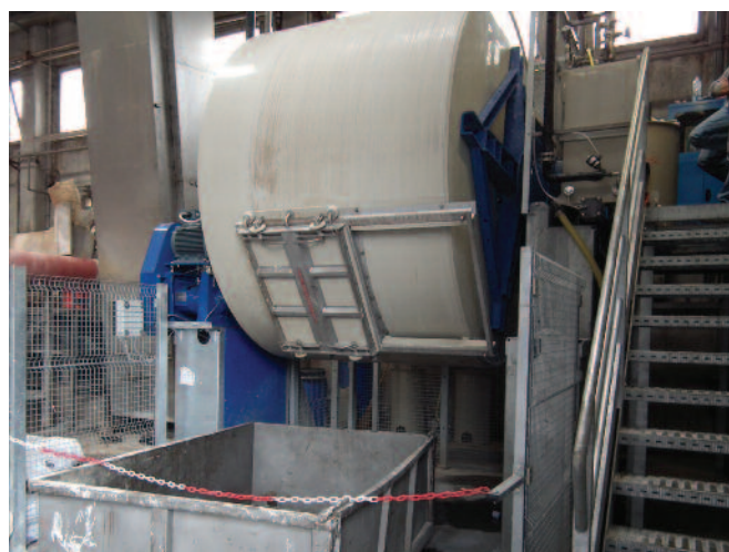
The Ecosmart Drum: This PPE drum has a double skin for a water jacket to enable very close temperature control. Two ton lots of hides for unhairing with hydrogen peroxide can be processed using this equipment.
