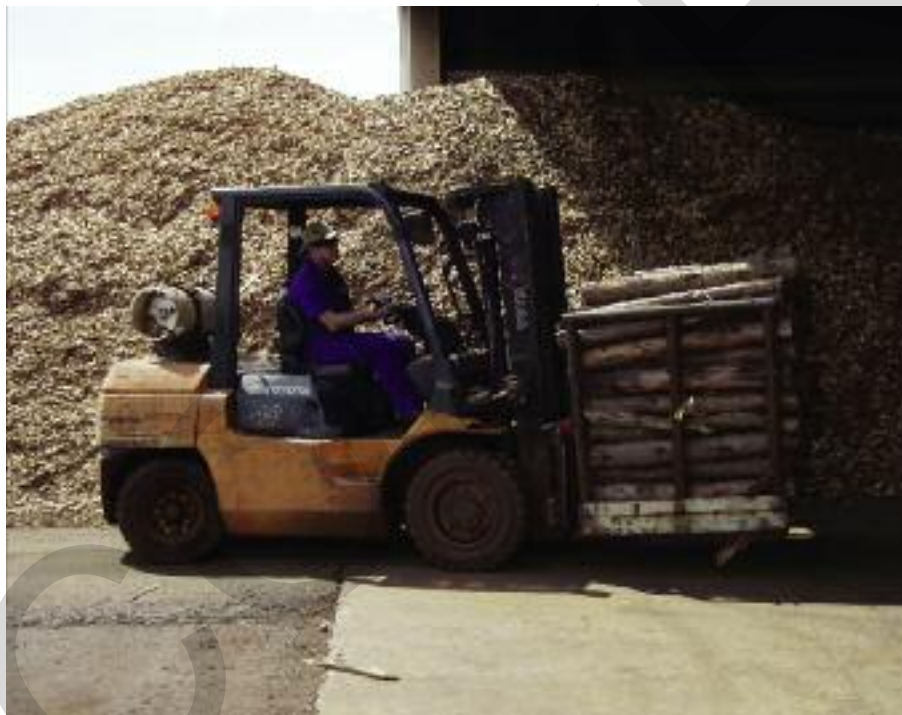
Pre-cut logs from renewable sources are used as fuel for steam generation. Wood from packaging and damaged pallets are also chipped and similarly used.
