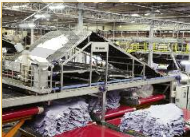
After samming, hides are delivered by belt conveyor for inspection, then automatic delivery to four grading platforms beneath the inspection unit that self-adjust for height. They are also fitted with conveyors that enable a load when complete to be moved forwards onto a holding station.
