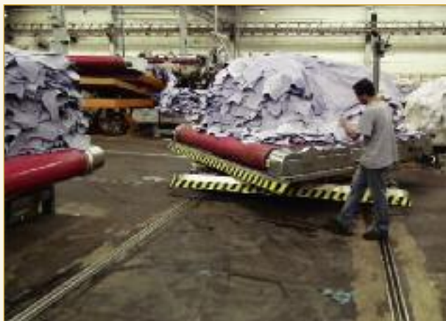
When required, a load is moved by conveyor from the holding station onto a robot set on rails. This robot can swivel the load, and automatically deliver the goods to the designated splitting operation.
