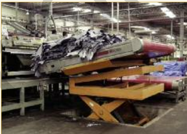
The robot delivers the load onto a holding station set next to the splitting machine before being transferred by the conveyors onto the jack. The load is rotated 90° for presentation, height adjustment and angled to optimise handling.
