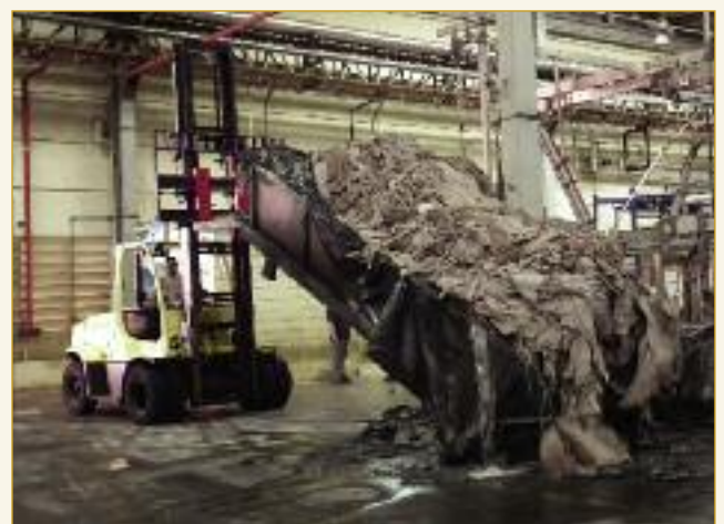
After dyeing the load, which can weigh up to 7,500kg, is dropped into a stainless steel container. Once tipped onto the floor adjacent the samm/setting machine, the hides are clipped on to a chain conveyor for delivery to this operation.
