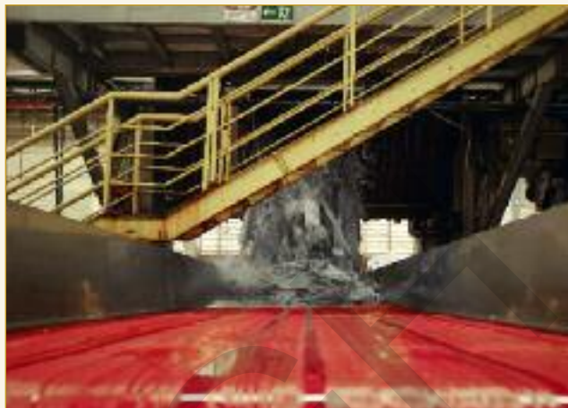
After a one hour wet back, the wet blues are dropped onto a stainless steel chute fitted with a conveyor to move the load forwards into a reception trough. They are then clipped onto a chain conveyor for delivery to the samming operation
