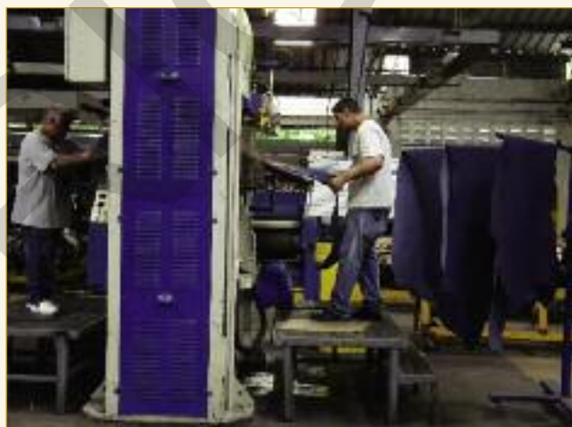
There are three ram presses used for plain and embossing effects. The production runs are managed to minimise plate changes, although this is rationalised to ensure rapid plate changes as required.
