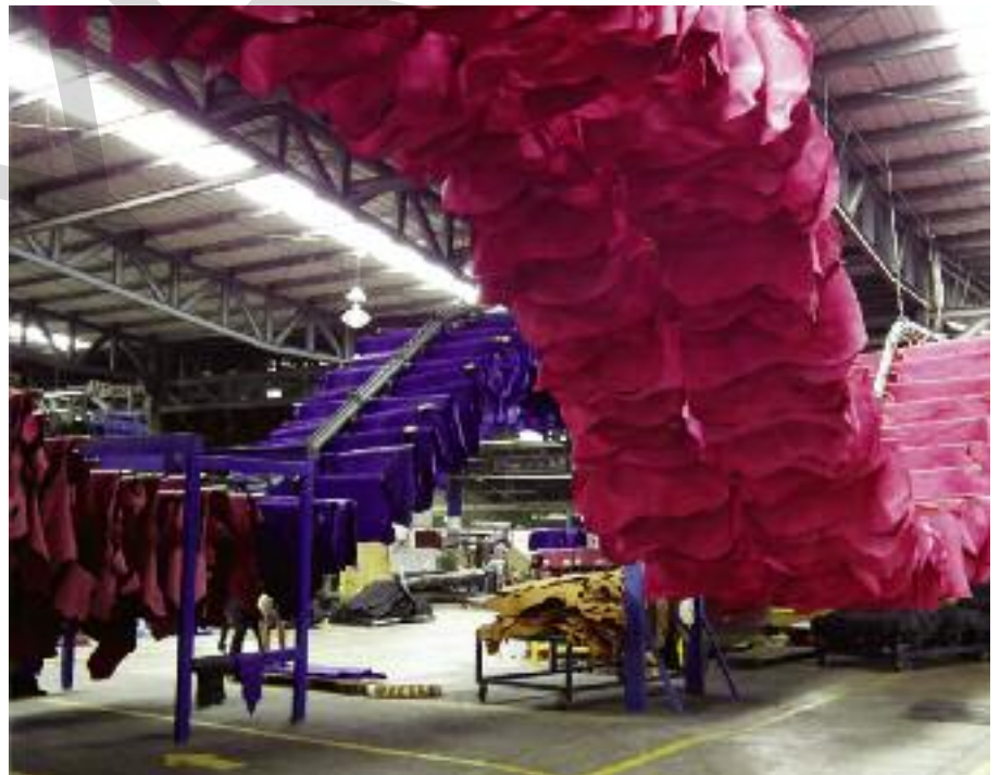
Leathers are mainly aired off after vacuum drying to finalise drying using overhead pole drying conveyors. The drying of firmer leathers also takes place using a TIAC unit.
