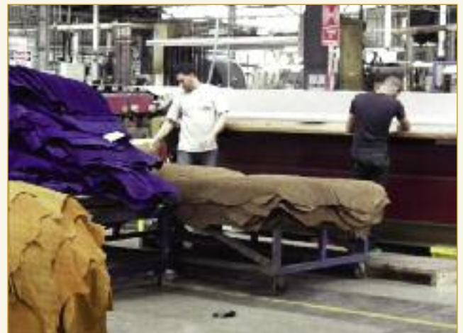
Shows the through-feed vibration staking operations which is used in conjunction with the seven tumbling drums.
