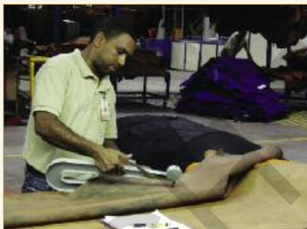
All of the leathers are checked to standard at crust sorting. Substance measurements are taken at six points across each side.
