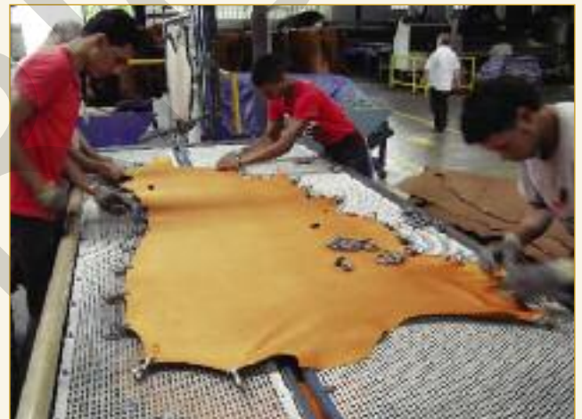
Leathers awaiting toggling are stacked behind the operative to the left. Dried leathers on removal from the frames are stacked to the right. This simple technique has improved the efficiency of leather handling.
