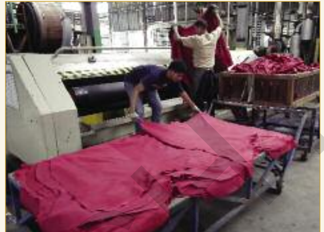
One of the two out-feed samm/setting machines as shown is dedicated to suede split leathers. The second machine is used for setting full grain leathers, and in conjunction with a through-feed Bause samm/setting machine.
