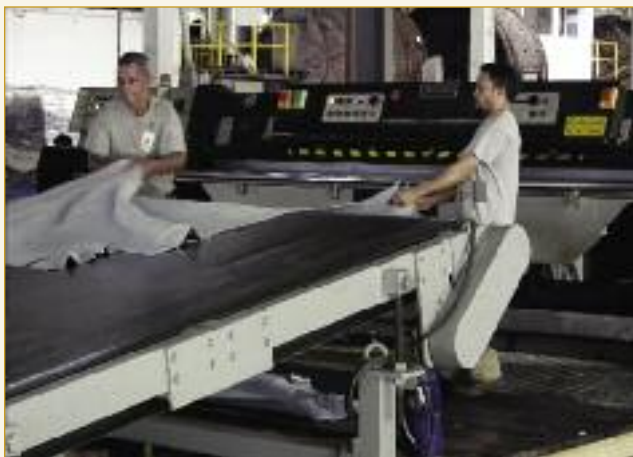
Hides are conveyor-fed to the blue splitting operation after samming flesh side up to maximise setting action. They are turned 90° for belly to belly splitting on Zebu hides to minimise damage to the hump area.
