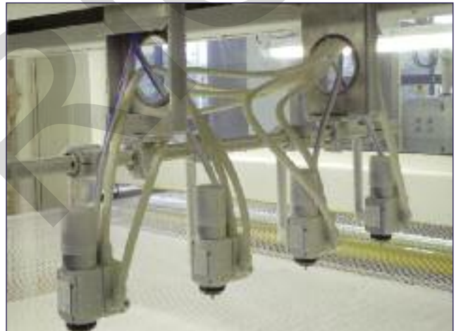
Four guns with air and product delivery connections.
