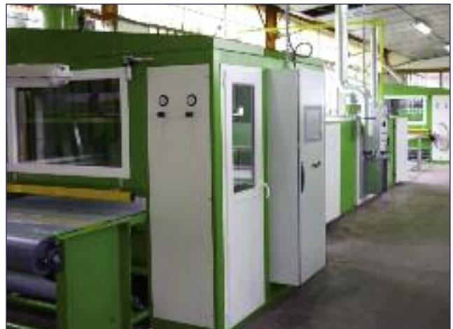
Reciprocator line with dryer and second sprayer.
