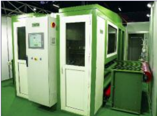
Side view of cabin showing touch screen panel for programming and control.
