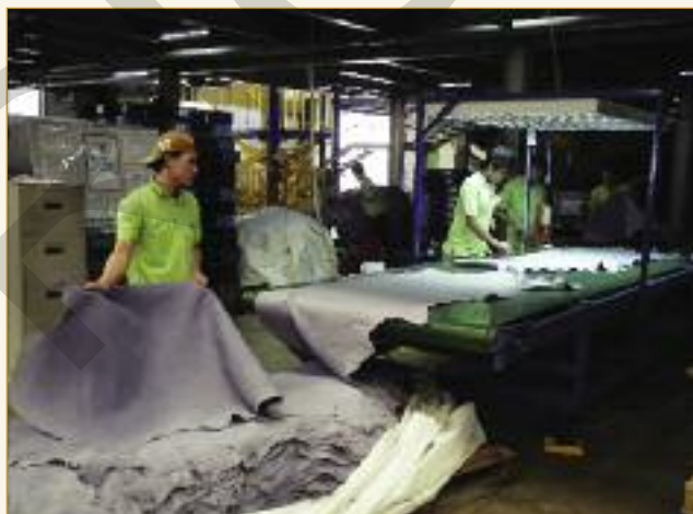
Blue sorting is performed under a series of lights on a moving belt. Leathers following splitting are stacked flesh side up, so that they can be easily turned over for the conveyor feed.
