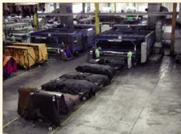
One of the three spraying lines within the finishing department. A mixture of gas and infra-red drying is used, and there is careful control of the moisture loss within drying operations to avoid area losses.
