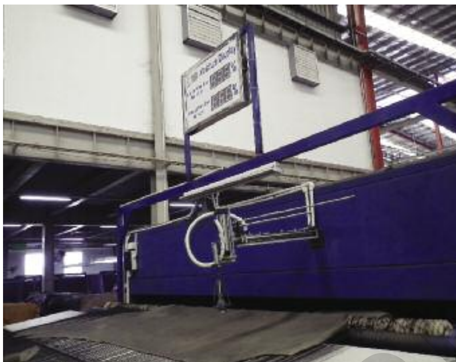
This equipment is designed to touch and measure the moisture content of each side as it exits the spray-drying cabinet. The moisture content for each side is displayed, and also the average value for the pack.
