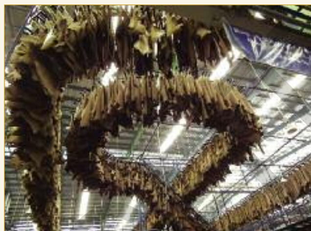
The drying operations are finalised with tension-free drying using overhead conveyors set in the roof areas. There are three drying lines that are used, and the leathers are dried to staking moisture content.
