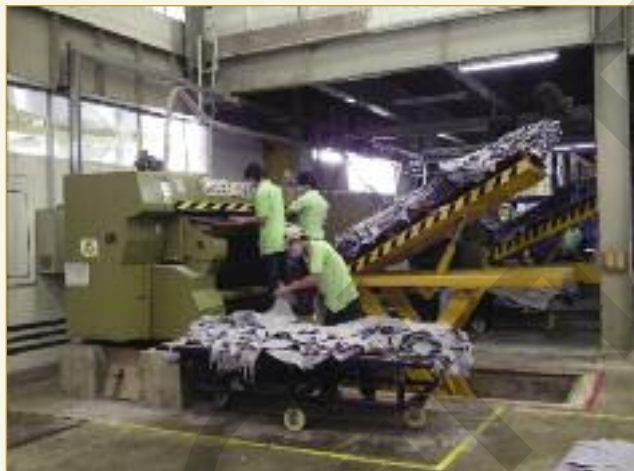
Each of the three shaving machines is operated by two operatives to minimise damage to the sides. The leathers are elevated and angled to reduce operative fatigue and improve the feed-off.
