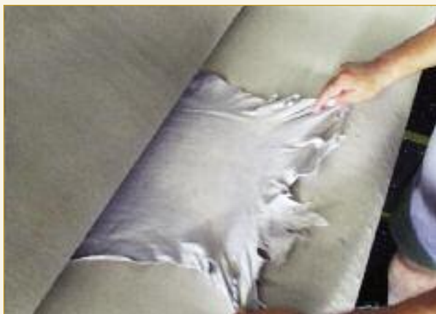
Because of the long neck and shanks, a degree of tangling is inevitable in processing. Although there is emphasis on samming to best present the skins, wet stretching and staking - as shown - is also employed to extend these parts for presentation to shaving.
