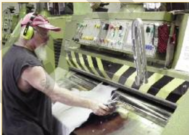
Shaving is an especially skilled operation when processing kangaroo skins as there is an unusually high need to manipulate the skins and extend the shanks and necks to avoid shaving damage
