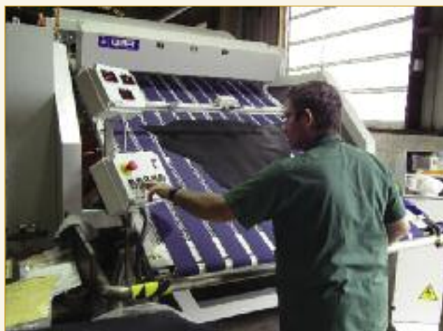
After final crust trimming, the skins are measured and graded, then automatically stacked according to grade before going to finishing.
