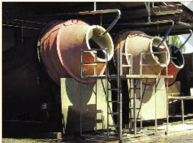
Canbar processors are used for processing kangaroo skins. For clear forklift access for loading and unloading purposes, a rail-track has been installed to move the elevated service platform to add chemicals and monitor the four vessels.
