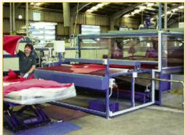
Top-coats are applied by spraying.
