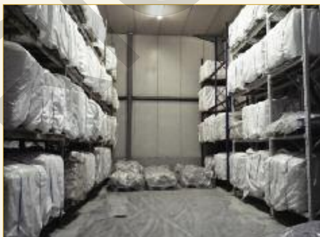
Kangaroo skins are first processed to the acid/salt pickled state, then held sealed in cold storage. This creates a buffer that is needed to overcome the considerable variations in supply and ensure a uniform input of skins to the tannery.
