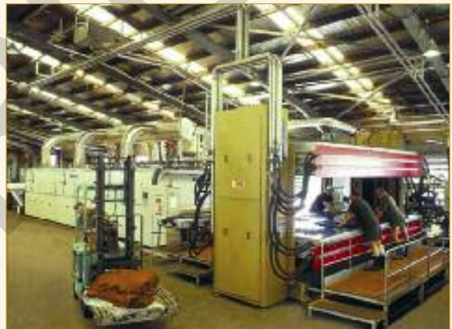
Vacuum drying is used to extend and flatten the skins before completion of the drying process using a horizontal through-feed drying cabinet. This dries the leather to staking moisture content, followed by feed into first-time staking.
