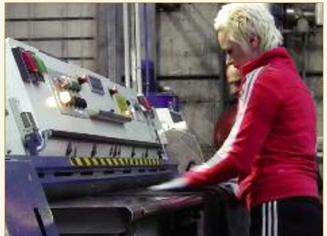
All of the leathers designated for steering-wheels are dry split for complete control of the leather thickness.
