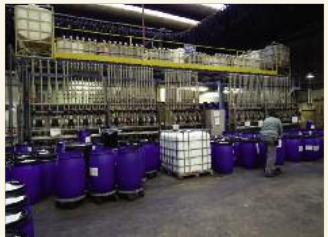
All of the finishing blends are managed using a dispensing system.
