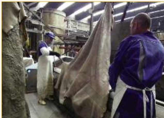
All of the fleshing is in the limed state as the processing operates to standards set down for food production. Hides are delivered individually to the elevated through-feed fleshing machine, the whole system being designed to minimise handling.
