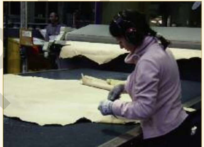
Softening is provided by combinations of through-feed vibration staking and dry milling both in the pre-finished state and within finishing. In this situation the pre-crust leathers are trimmed on a conveyor after staking. Operatives wear ear protectors.
