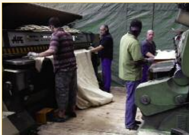
Hides are delivered fully opened from grading via over-machine conveyor for shaving. The butts are shaved on the first machine, then passed to the team on the second machine for shaving the necks. All machine settings are controlled from the first (master) machine.
