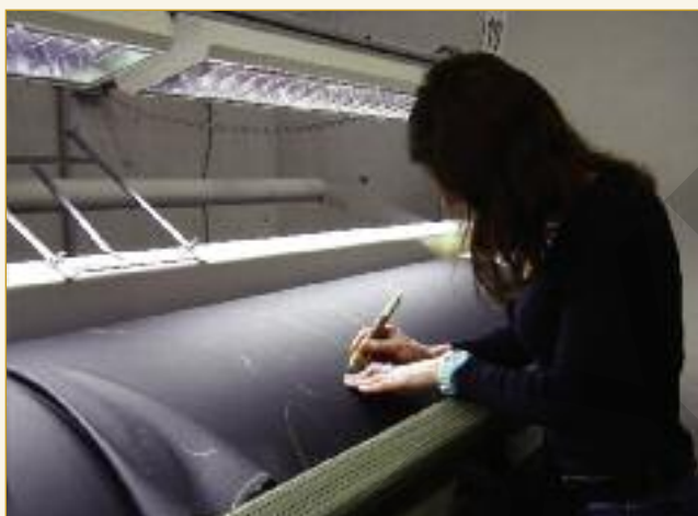
After an initial hide inspection, and identification of defects, the hide is stretched by 5%. Hidden defects are revealed, and marked according to a colour code.
