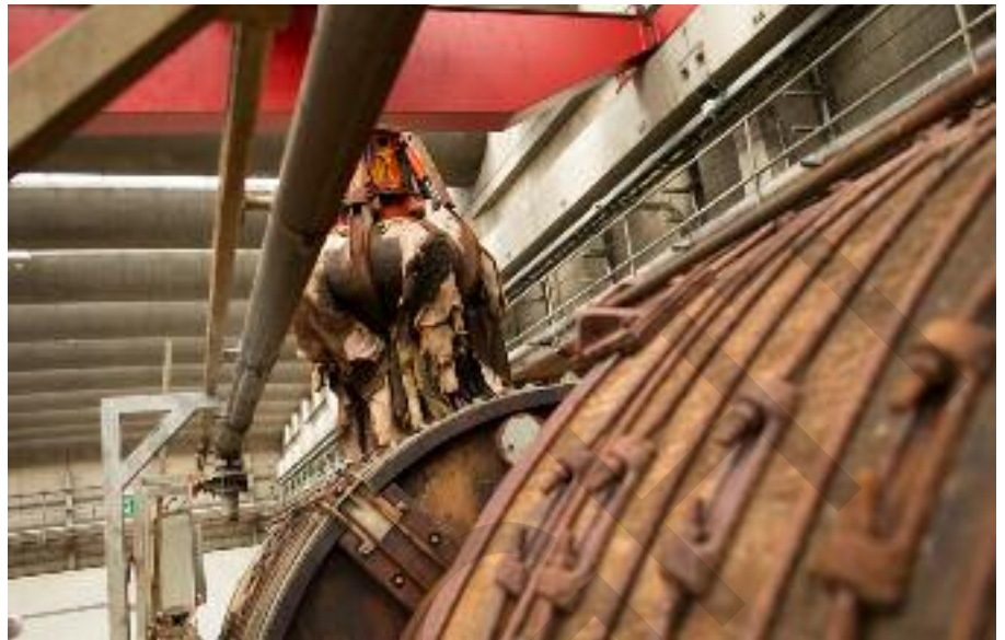
The movement of materials in the wet processing areas is highly dependent upon hoists operated from overhead cranes that run on parallel rail track set beneath the roof. These tracks run the whole length of the wet processing areas for moving hides both by grab and stainless steel containers.
