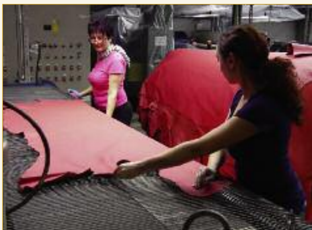
Many different colours are produced to cover the range of leathers manufactured. Close attention is paid to ensure removal of any dust within finishing operations.
