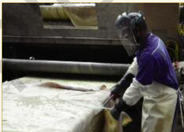
After lime splitting the flesh splits are trimmed to remove bellies and necks to provide uniform coupons for split manufacture. Particular attention to safety requires full face guarding against possible knife cuts, and eye protection against possible splashes.
