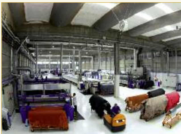
The humidity and temperature is controlled within the finishing department to avoid variation and help control the absorbency of the grain of the leather within finishing.
