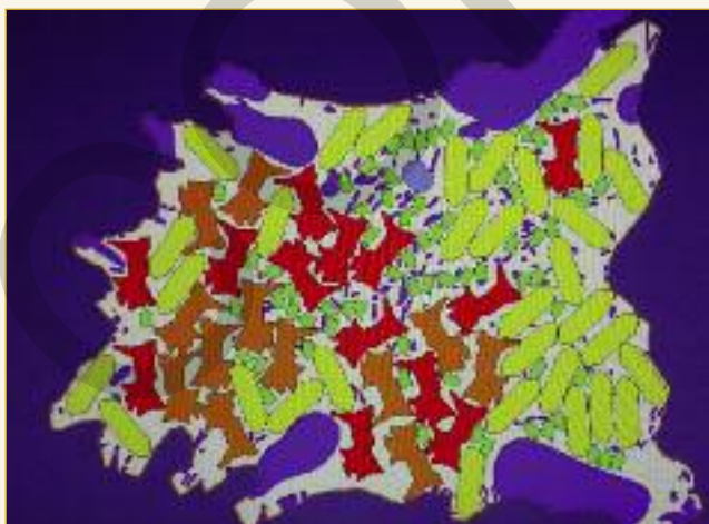
Within the cutting plant, the leather is scanned, and the cutting arrangements for the steering-wheel components optimised by computer. This takes into account both the pre-marked defects identified in the tannery, and the direction of minimum stretch as required the final component.
