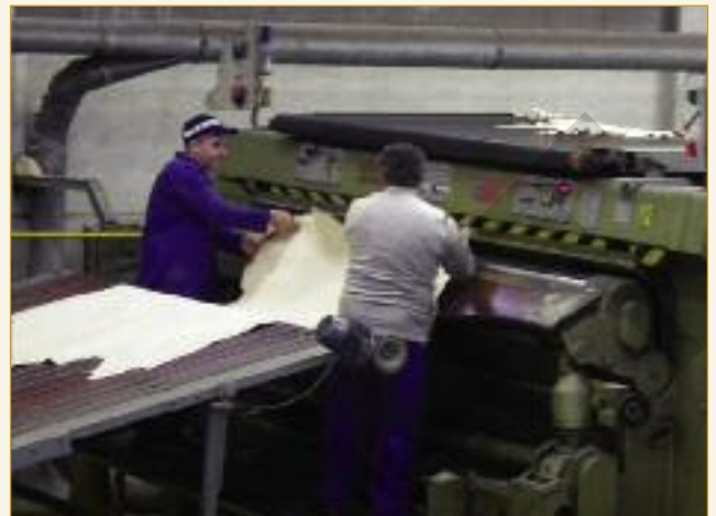
After samming, the fully opened hides are delivered flesh side up for direct feed to the shaving operation. After shaving, the hides exit over the top of the shaving machine by conveyor, grain side up for inspection and grading.
