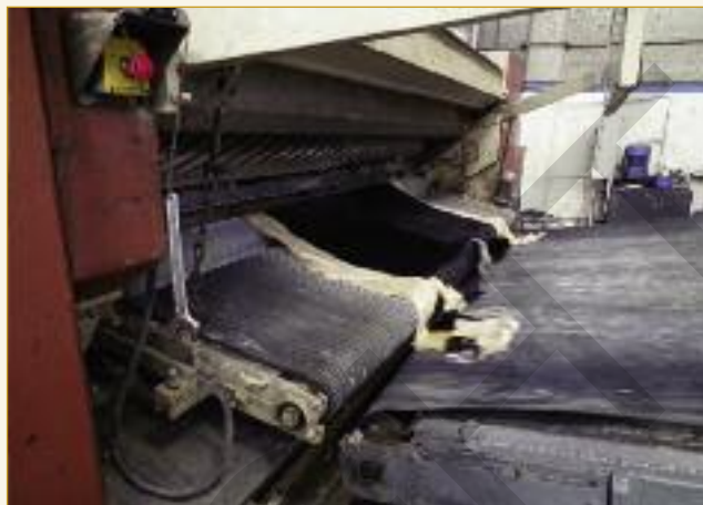
There is considerable focus on the fleshing operation before unhairing/liming as none of the hides that are processed are lime split. The photo shows out-feed from the through-feed fleshing operation.
