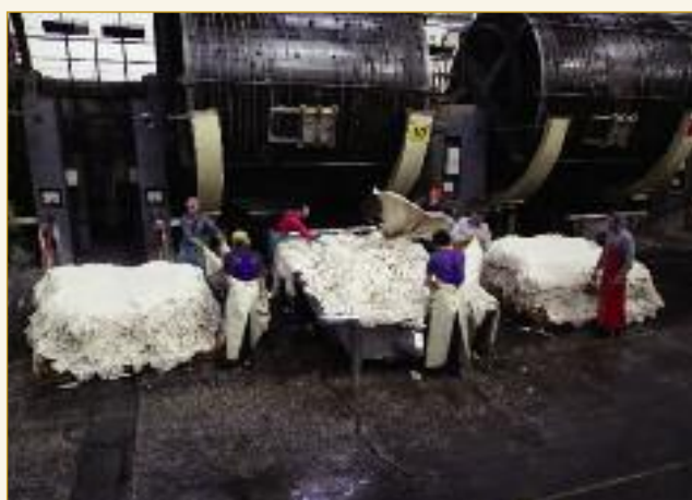
After a chrome-free tannage the hides are dumped into stainless steel trucks, then stacked flat onto two stillages in preparation for samming the following day.
