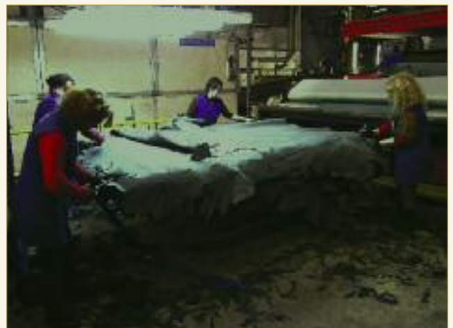
Within a team of four, hides are simultaneously trimmed by two people and graded by the other two team members. Once graded the hides are slid into the feed for through-feed vibration staking.
