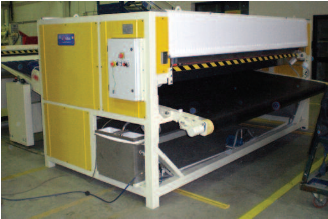
The dedusting machine removes dust from the grain before or after finishing.
