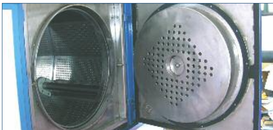
Access door open showing internal rotating drum configuration with one of its shelves.
