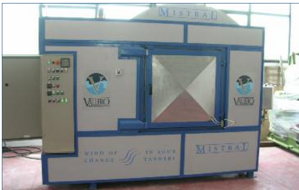
Front view of the Mistral with access door closed. Control panel with display screen is seen on the side of the machine.
