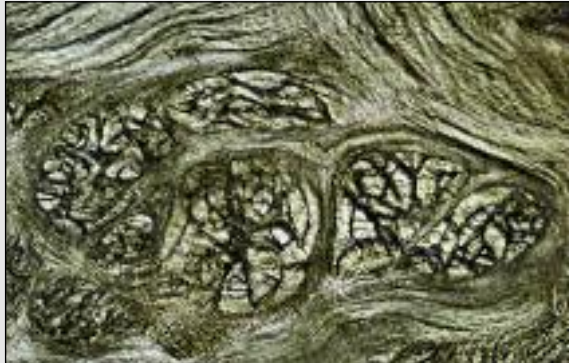
Panel 3/3a: Shows a poor opening-up of the fibre structure
