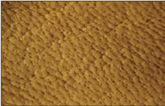
Panel 3/2a: Grain surface showing good grain break (aniline calf)
