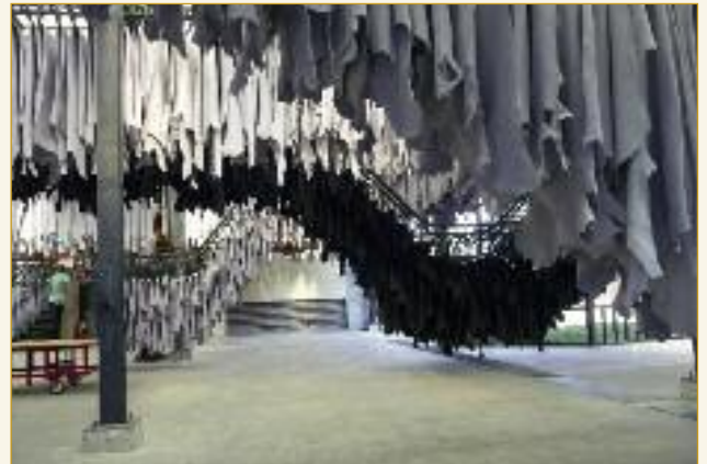
Part of the pole-drying unit for natural drying of all leathers after vacuum drying.
