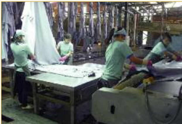
Wet blue are opened, inspected and graded by the four operatives on the stainless steel table, then slid forward into the samming machine.
