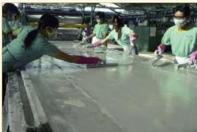
Finish is applied to pigmented leathers using a felt covered roller. The finish is then hand padded by the team onto the leather to ensure good adhesion and even coverage.
