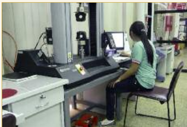
The Instron test for tensile strength is among the routine tests performed in the finished leather assessment laboratories.
