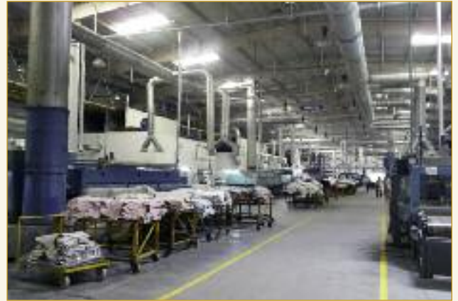
One of the two finishing departments. This one is used for finishing sheepskins and light coloured leathers.
