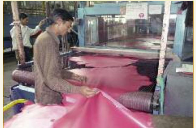
One of the spraying machines for sheepskin leathers. The steam drying cabinets are to be replaced with infrared drying cells to reduce energy demands.
