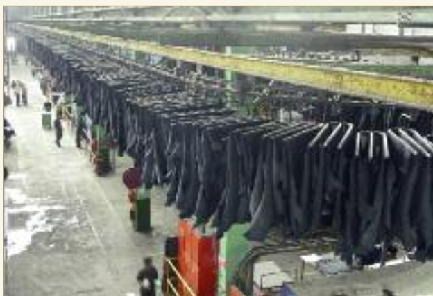
The pole-drying unit is used to provide a natural air drying for soft leathers.
