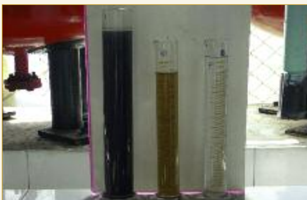
Examples of effluent after primary settling, the effluent after conventional physical and biological treatment, and the permeate after reverse osmosis. This water is suitable for re-use in leather processing.
