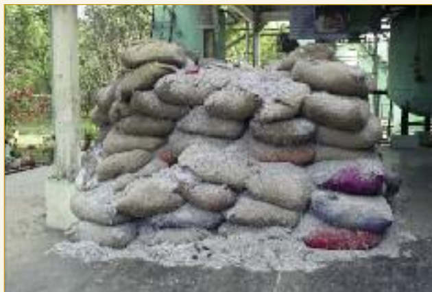
A single day's production of shavings awaiting processing to produce collagen hydrolysate, and chromium hydroxide as part of the recovery of chromium sulfate.
