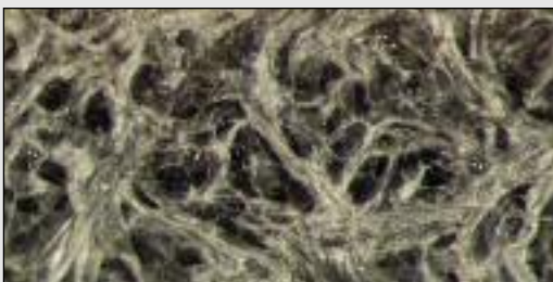
Panel 2/4a: High angle of weave typical of tension-free drying
