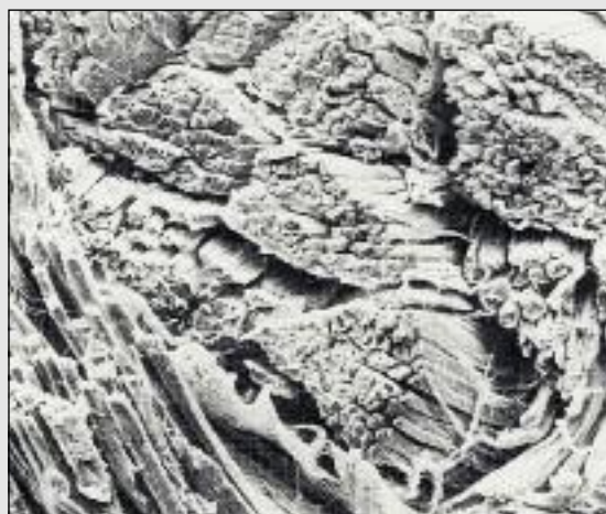
Panel 2/1b: Fibre structure: large splitting up
