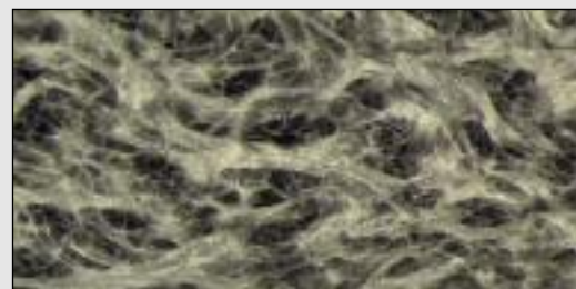
Panel 2/4b: Lower angle of weave typical from drying under tension
