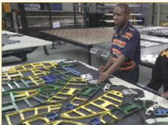
The hides are marked according to the quality differences across each hide, and the colour-coded cutting dies are placed to maximise yield. The cutting board holding these hides can be readily moved from the work tables for feed to the cutting presses using a combination of ball and roller bearings.
