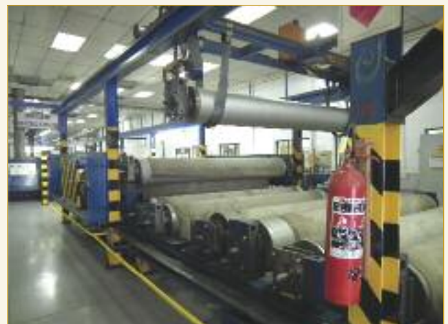
25 embossing rollers provide a wide texture range for Seton. Four embossing machines are set in line in a custom-designed servicing system that enables all embossing rollers to be changed with minimum downtime.
