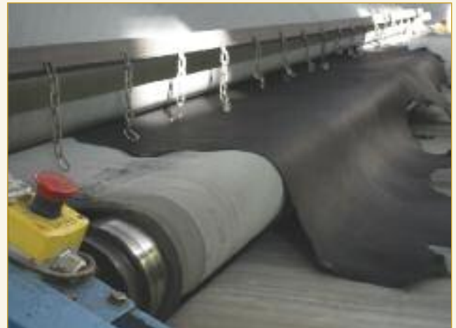
Static electricity causes fibres and dust to remain on the leather after staking using three feed-through vibration staking machines set in tandem. Steel chains are set at the out-feed from the final staking machine to remove charge from the leather and ease fibre removal.
