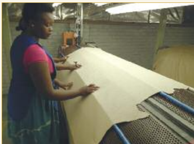
Inspection is central to product assurance, and this is performed by holding leather under tension on rotating frames. The inspection and identification and marking of defects is time-consuming, each hide inspection requiring on average five minutes.
