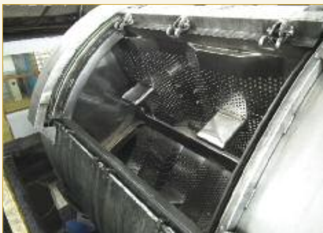
All of the dyeing and retanning operations are performed in 12 stainless steel tri-compartmental Dose vessels. These are of two sizes to accommodate two different input weights and apply the same level of mechanical action.
