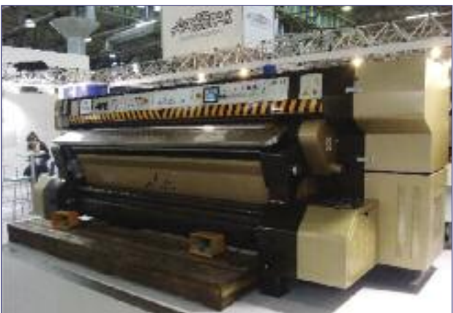
Alpespak Suprema wet blue splitting machine with dual operator controls.
