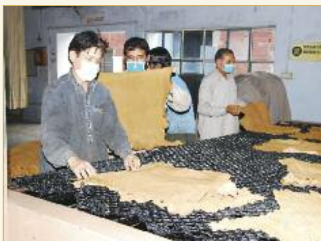
Special mesh on a spray-coating machine to prevent small skins from slipping through.
