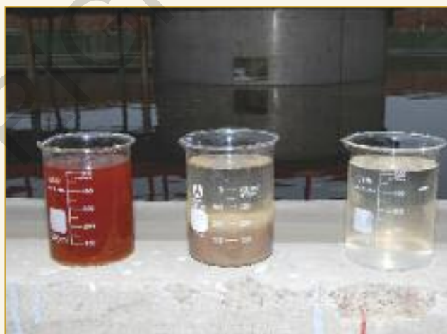
Before, during, after. Water from the wastewater treatment plant is clean enough to go back to the tannery for re-use in production.
