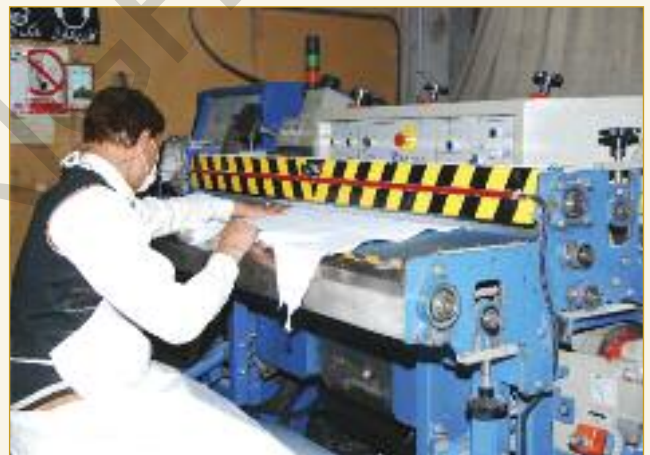
A new Alpe splitting machine will help the tannery cope with an increase in bovine hide production.
