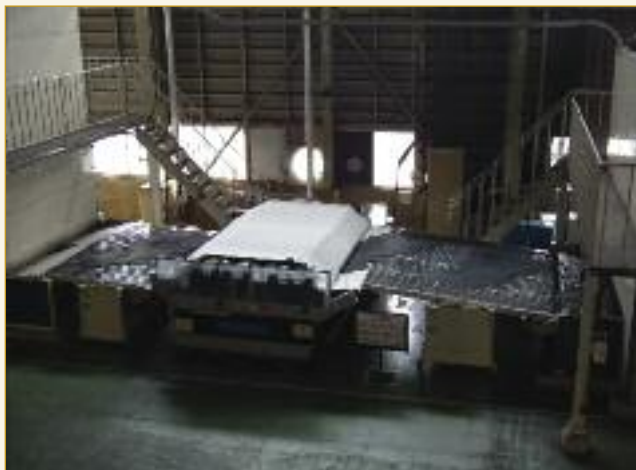
After samm/setting and vibration staking, the leather is dried using two throughfeed drying tunnels. These are separated by a second wet stretching machine to soften and extend the part dried leathers.
