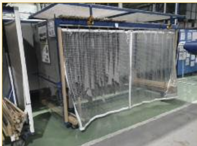
Leathers throughout the finishing department are carefully managed to avoid contamination. This shows the moveable holding racks that are loaded at the end of spraying operations, where the leathers are protected by plastic curtaining.
