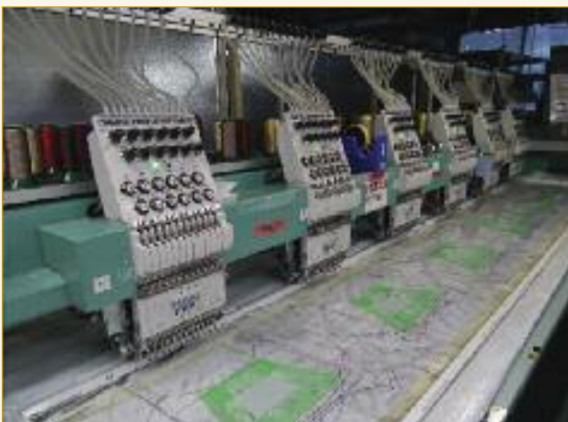
Very intricate stitching is required to create patterns and details on many automotive components. This computer managed system was installed in 2009.
