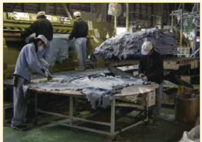
Shaved pieces are dropped onto these circular tables for trimming. These can be rotated to ease the trimming operation for the operatives.
