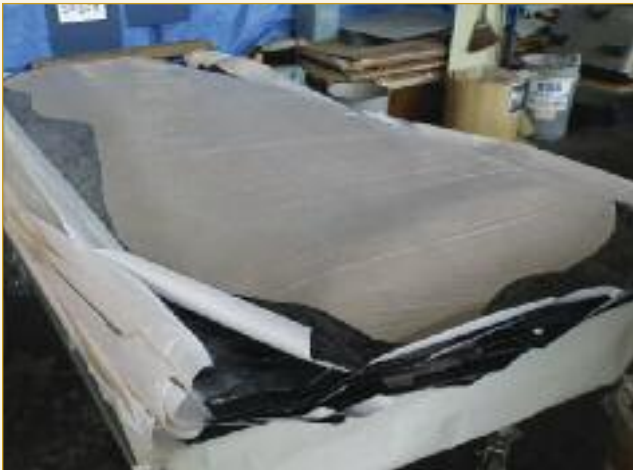
This shows leather placed onto cast finish films that are still attached to backing paper. After heat lamination, the paper is peeled from the finish to reveal the slightly embossed grain surface.
