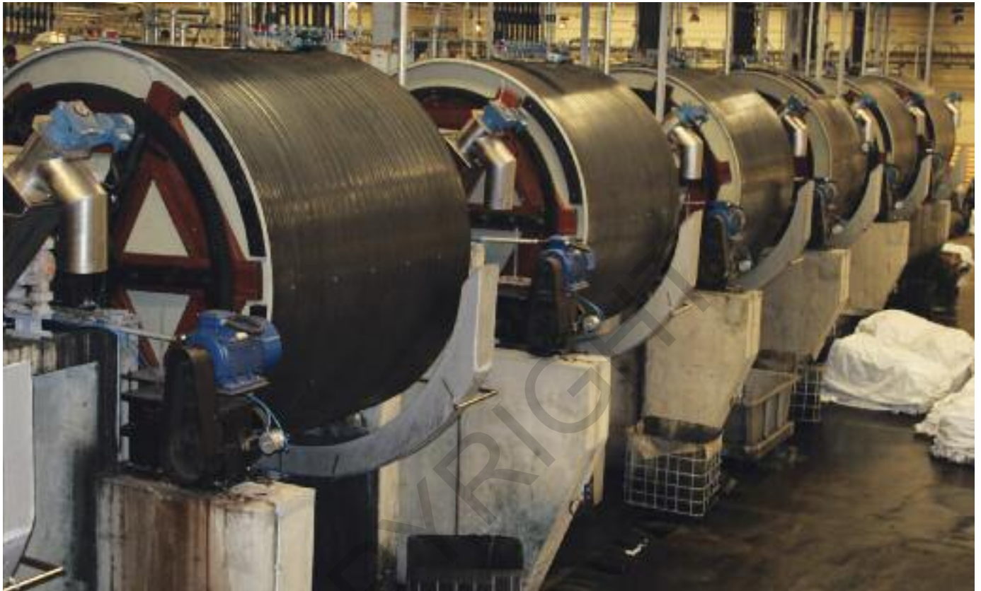
Jumbo polypropylene PPH drums, note absence of external construction elements.
