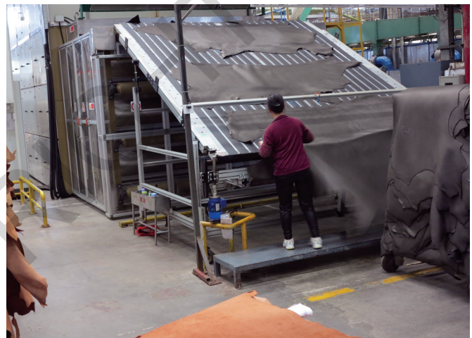
Cartigliano conditioning unit being fed manually.
