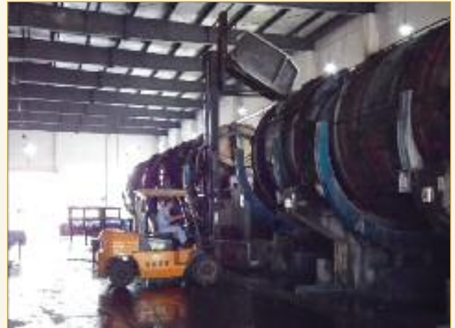
The major movement of goods within this plant is reliant upon forklift trucks, as shown loading one of the tanning drums.
