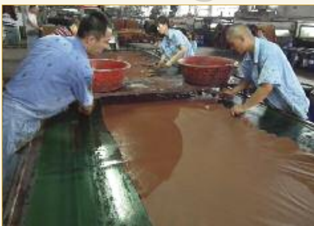
Another example of hand operations is the first finish coat application. It is considered that this ensures a more individual attention to the needs of each piece and a higher base coat adhesion.
