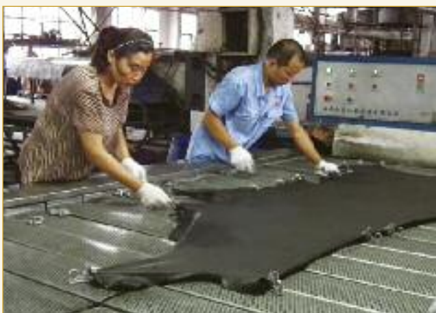
Toggle drying is also employed, and takes place following dry milling both before finishing and within finishing operations.
