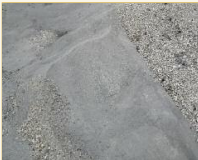
Combustion within the coal fired steam generation plant is very efficient, as demonstrated by the fine ash which is virtually carbon-free.
