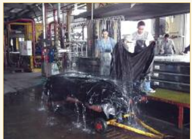
Before vacuum drying the pieces are sprayed with water to assist the hand setting operation. This water is continuously collected, screened and recycled back to the operation.
