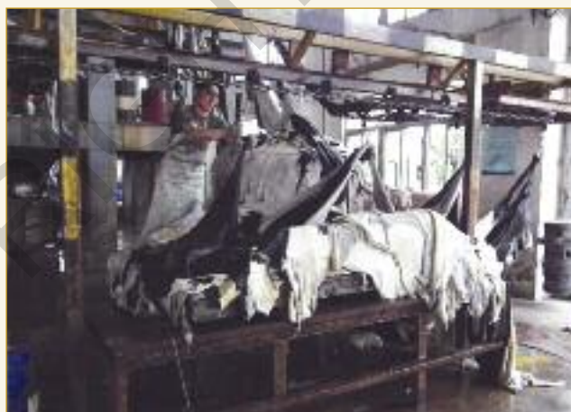
These Australian hides have been lifted by forklift onto the loading station for attachment to a conveyor line that feeds the elevated fleshing operation. This arrangement is used on all three pairs of fleshing machines.
