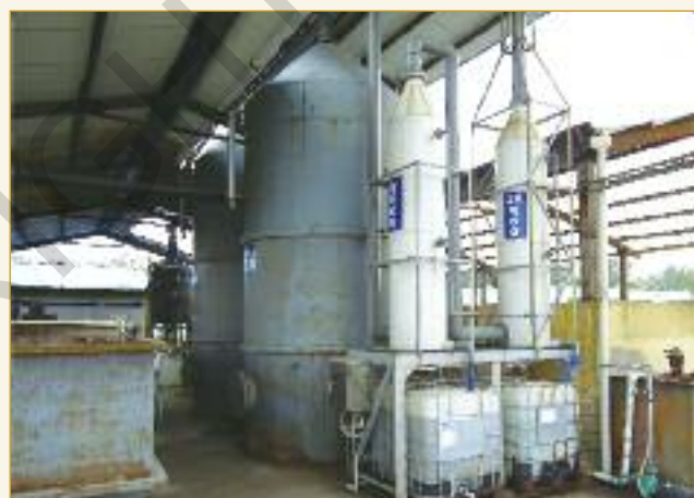
Hydrogen sulfide is liberated from the used lime/unhair liquors by acidification in the two sealed tanks, and the gas washed into solution in two scrubbing columns. Sodium hydroxide solution is used as the wash medium, and the recovered sulfide is used in subsequent liming/unhairing processing.
