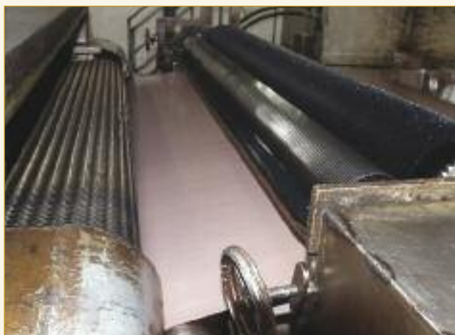
This photo shows the interior of the oil swabbing machine. After heating the leather grain using infrared heaters, the leather is roller-swabbed with hot oil. The level of offer is controlled by the machined roller that offers precise quantities of oil to the swabbing roller.
