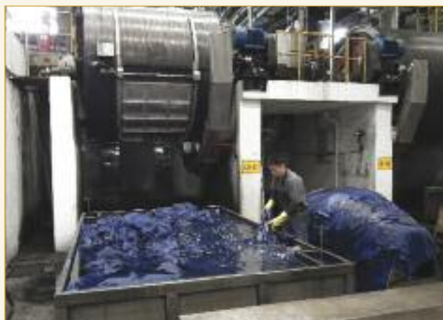
After dropping the load from the new deep shelf drums into trucks, the sides are individually stacked and placed on stainless steel horses.
