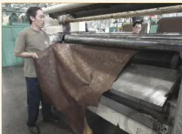
There are two Starprint machines by Gemata that create a variety of tipping effects on oiled leathers.
