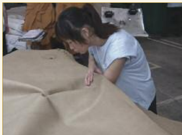
All of the leathers are inspected in the crust condition. There are four teams in total, and each comprises four people; the teams inspect every side for grain break.
