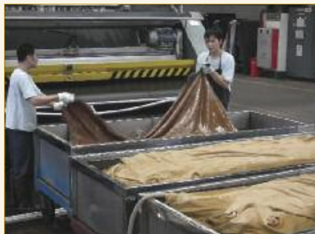
As part of coloured samm/setting, the sides are removed from stainless steel troughs and floated with water to avoid compression. This operation is followed by wet staking/stretching.
