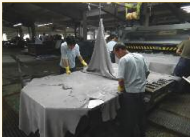
All of the wet blue stock is soaked until fully wet back. After unloading from the paddles and drums onto the floor area, they are hooked onto a line conveyor to the samm setting operation where they are opened in preparation for machine feed.
