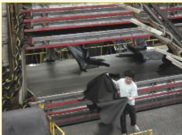
Vacuum drying is an alternative drying method that is employed following samm/setting and wet staking. After partially drying, the sides are placed onto a pole conveyor for the final drying phase.
