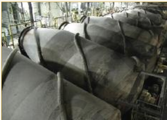
Part of the back-to-back rows of hides processors used for soaking and liming. Each processor operates with an input weight of 14,500 lbs on a two day soaking/liming/unhairing cycle.
