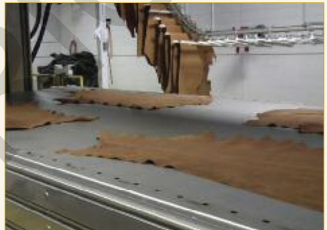
All of the leathers offered to the vacuum drying plates have been wet stretched/staked after samm setting. These sides are well extended, and can be simply placed on the plates without the need for any hand setting.
