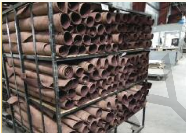
Leathers for delivery to Red Wing Shoe are individually rolled and placed on racking suited for direct use within the shoe factory.
