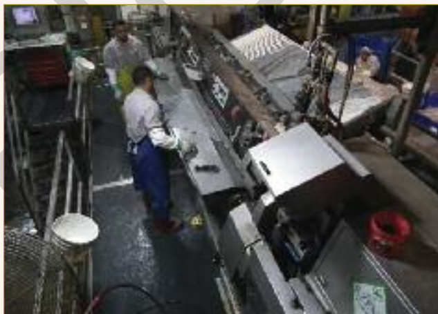
All the hides that are contract tanned for SB Foot are lime split. The grain splits are tanned in conventional Vallero International tanning drums, with the trimmed limed splits being sold for collagen manufacture.
