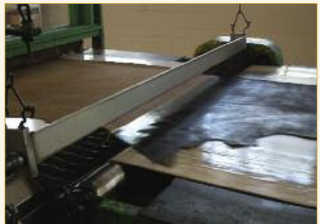
Leather is curtain coated on the grain and flesh sides with specially blended oils as the first stage of finishing. The curtain coating machine is suspended on rubber mountings to eliminate disruption of the curtain due to any vibration.
