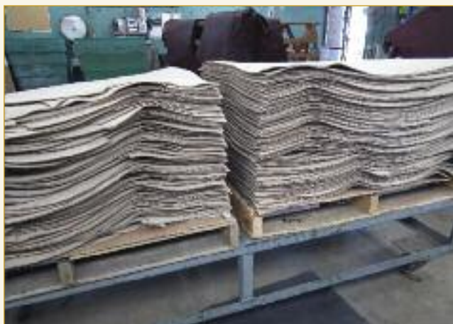
These sides are cut in two to customer specification. These leathers are impregnated with resin, then dried, and are used in mechanical applications in ultra-cold conditions experienced in Canada, Russia and Alaska.
