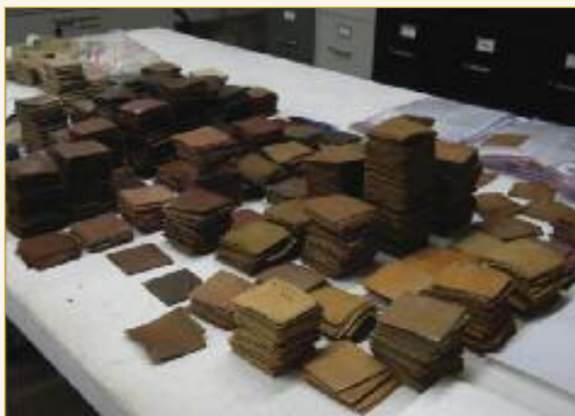
Cuttings are taken and dried from each pack of leather at the end of dyeing/retan/fatliquoring. Placed on top of cuttings from previous packs in the control office, this presents a detailed colour profile of production and, by comparison to other packs and master samples, is central to basic colour management.
