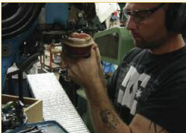
After closing, the upper is lasted and a welt sewn in using the Goodyear welt process ready for the soles to be attached.
