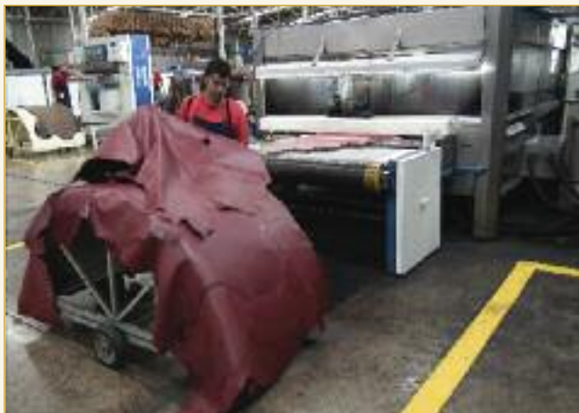
There are four spraying machines used for finishing. One machine is installed in a separate department and used for finishing white leathers only.
