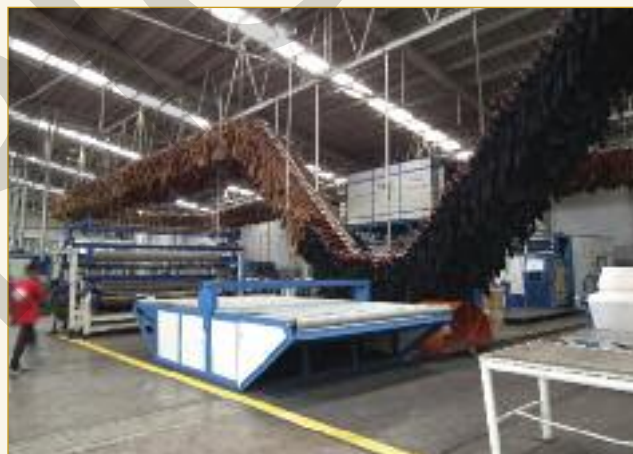
All of the leathers are aired off after vacuum drying. This operation is supported by forced air drying within cabinets enclosing part of the conveyor line if required.
