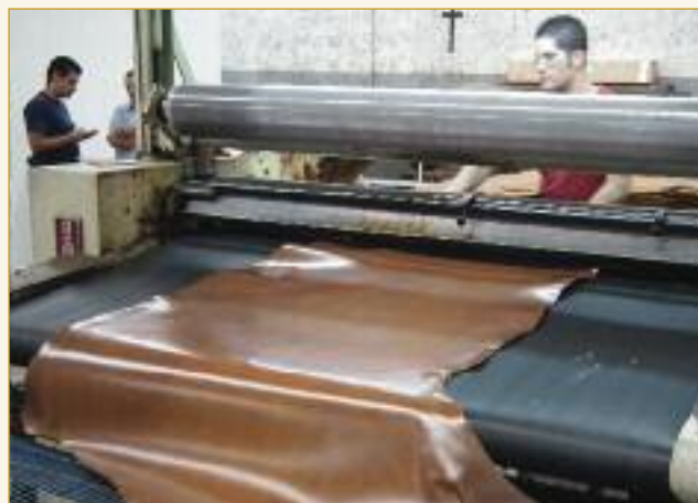
Hot waxes and oils are applied to about 25-35% of the leathers in finishing by roller coater.
