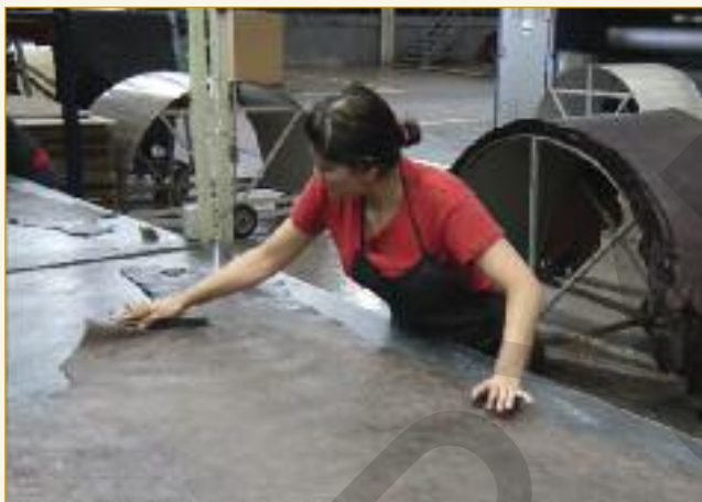
Many different effects are developed by combinations of finish applications and milling. In this example, part finished leathers are being stressed by hand.
