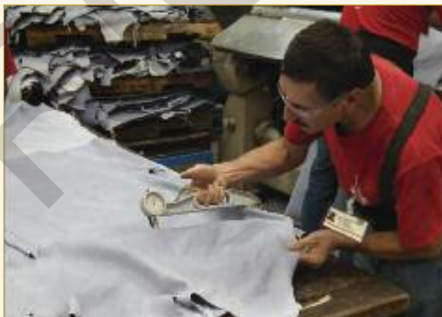
On shaving, every 10th side is measured for thickness in areas specified in the production manual. Machine adjustments are made as required based on these measurements.
