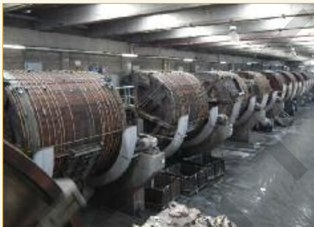
The soaking/liming and tanning drums are set in an L-shape within Curtec, and serviced by a rear mezzanine. All chemical additions are made manually, with automatic water supply.
