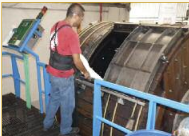
All of the chemicals are weighed and added to the drums manually in the dyeing and retanning area.
