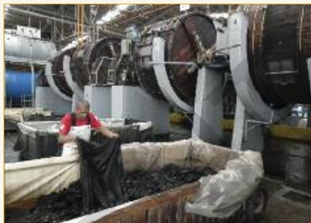
After retannage/dyeing, the sides are discharged into containers, then manually stacked before offer to the samm/setting operation.
