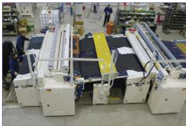
Overview of Wet-Wet line coating machines (1) and (2)
