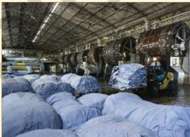
In the beam house and tanning departments there are 6 Vallero wooden drums which operate with a raw input weight of 6 tonnes per load. The tanning drums are fitted with heating systems which are used to improve the uptake of chrome in the tanning process.
