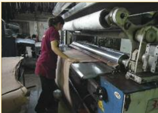
Both the chrome and the vegetable tanneries have their own finishing departments. Both are fully equipped with roller coating machines, spraying machines and roller presses and embossing machines. These are not linked together as there is a wide variety of leathers being manufactured at any one time.
