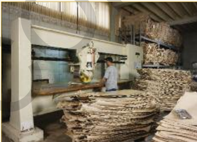
In the final stages of manufacture, the croupones are measured for substance, then rolled to compact the fibre structure. This machine is fully guarded, and will only operate with the operative standing on a pressure sensitive plate.
