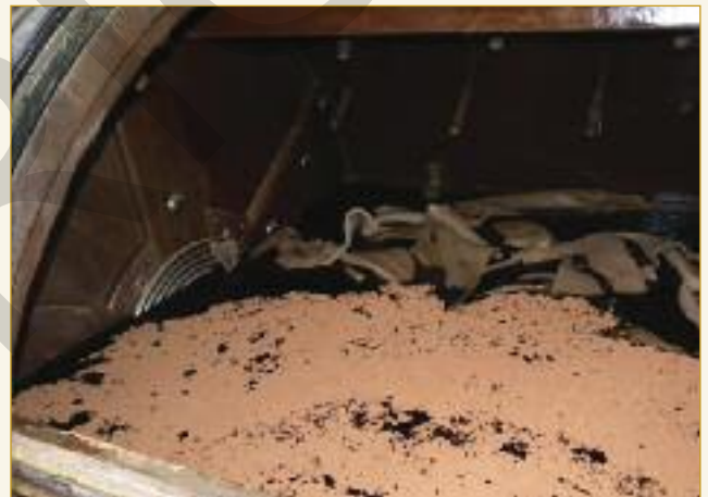
Billeri drums are used after 14 days in the pit system for the final tanning stage. This stage takes three days, and mimosa, quebracho and chestnut extracts are added to this bath to maintain the tannin concentration of the float.
