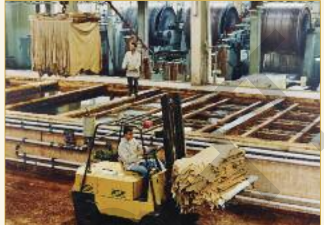
Pieces undergoing pit tanning as the first stage of sole leather tanning. The pieces are regularly raised on the frames to avoid prolonged contact between pieces, thus avoiding colour variation and ensuring uniform penetration of tannins.
