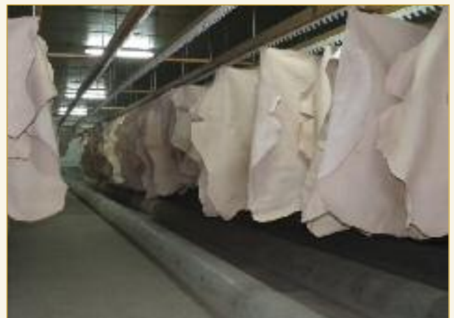
The sole leather and vegetable tanning tanneries are managed independently to avoid any contamination and avoid staining. A slow and controlled drying over a period of three days is needed for drying these vegetable tanned sides.
