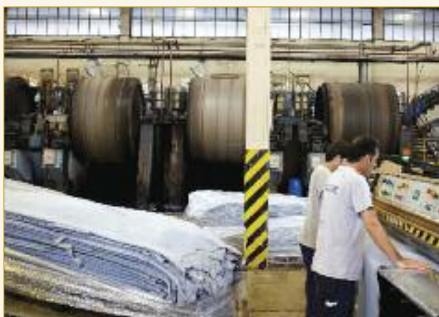
The splitting machine employs an elevated table for optimum feed to the splitting machine. The machine is fitted with a dust extraction unit to collect and scrub the dust generated at knife point by the operation.
