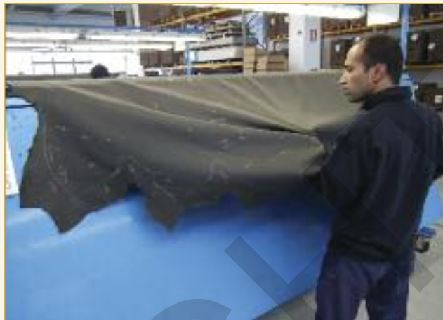
Dani Automotive Tannery: After careful assessment, cutting dies are placed onto leathers designated for steering wheels. The quality variations across the hide have been identified and graded. The cutting of components for automotive seating is automatically managed according to the cross-hide quality ratings via computer control.
