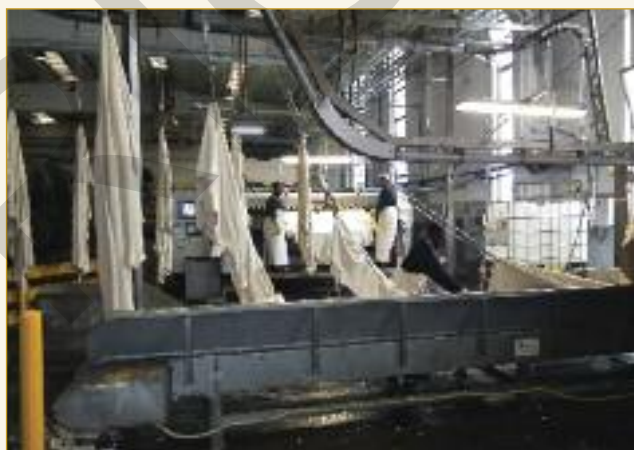
Dani Automotive Tannery: After tanning, the wet white leathers are moved to the sammying area where they are hooked into a chain conveyor for separation and feed to the sammying machine conveyor for grading, sammying and stacking as assessment.
