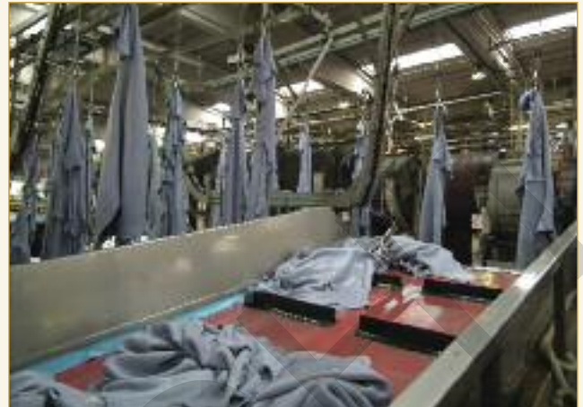
Dani Tannery: After wet blue tannage and grading and samm/setting, the hides are fully sealed with polythene and held in store. After drum wet back they are discharged onto a belt conveyor, then clipped onto a chain conveyor for delivery to samm/setting.
