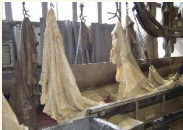
Developments: Oxidative unhairing. Hides following this sulfide free unhairing technique can be compared to the hides from the standard unhairing liming process that are also suspended from the chain conveyor.
