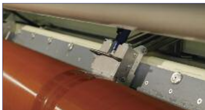
Cleaning device completing second cycle. Wastewater/Chemicals mixture is seen behind the device
