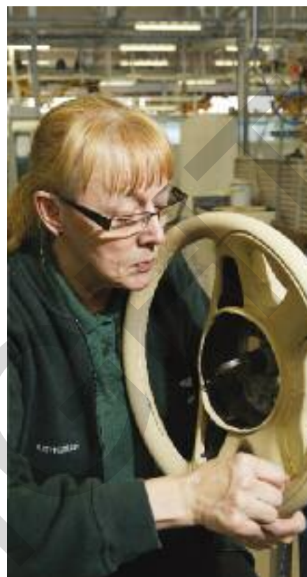
The company stitches by hand the leather covers on its steering-wheels. Each cover can take two days to create, or even more if the customer wants cross-stitching.
