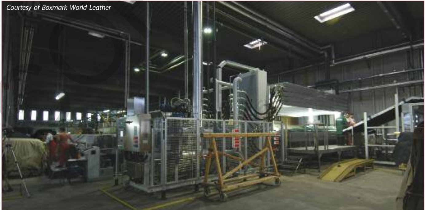
Sheepskins throughfeed drying line composed of wet stretching, conditioning unit and staking machine. Capacity of this line: 1,380 skins per hour. Courtesy of Dongming Bright Leather.
