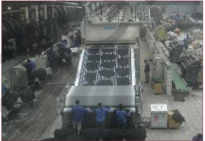
Sheepskins throughfeed drying line composed of wet stretching, conditioning unit and staking machine. Capacity of this line: 1,380 skins per hour. Courtesy of Dongming Bright Leather.
