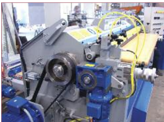
Aletti buffing machine type SV1800 which employs a buffing cylinder. Its control systems and performance are similar to the abrasive endless band type machines.
