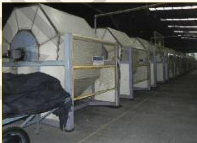
Line of milling drums. There are more than 50 milling drums on site used to create various finishing effects.
