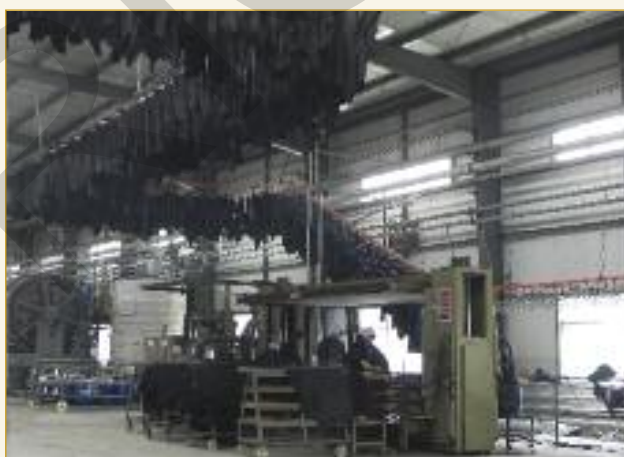
After vacuum drying, the pieces are placed on the overhead pole drying conveyor to complete the drying operation.
