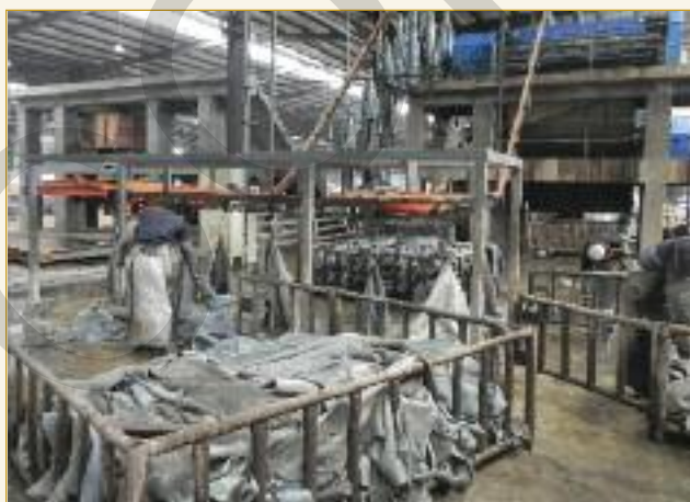
The limed hides are hooked individually onto an overhead feed conveyor to the fleshing operatives.
