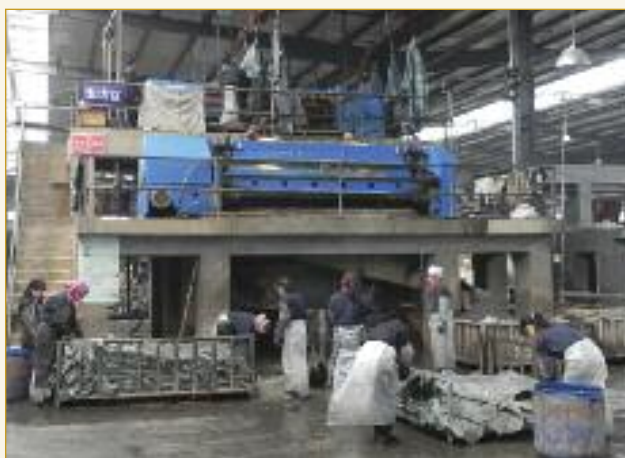
The fleshing machine is elevated, and the fleshed hides are loaded into containers and moved from the area by the fleshing team.
