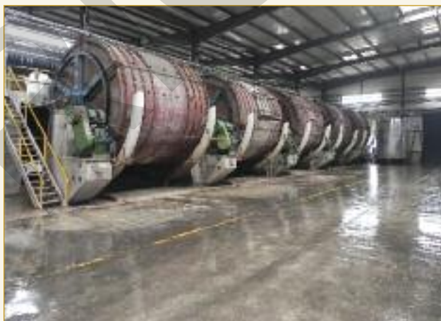
There are 20 drums in total being used for soaking and liming. All of the movement of raw, limed and chrome tanned leather is based on forklift trucks.
