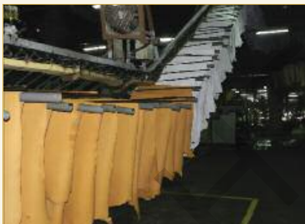
After vacuum drying, the sides are aired off by suspension drying on the overhead conveyor system that runs within the factory roof areas.
