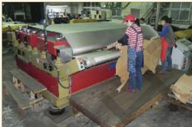
The moisture content of the drying operations is carefully controlled, and all of the leathers are staked using a feed through staking machine.
