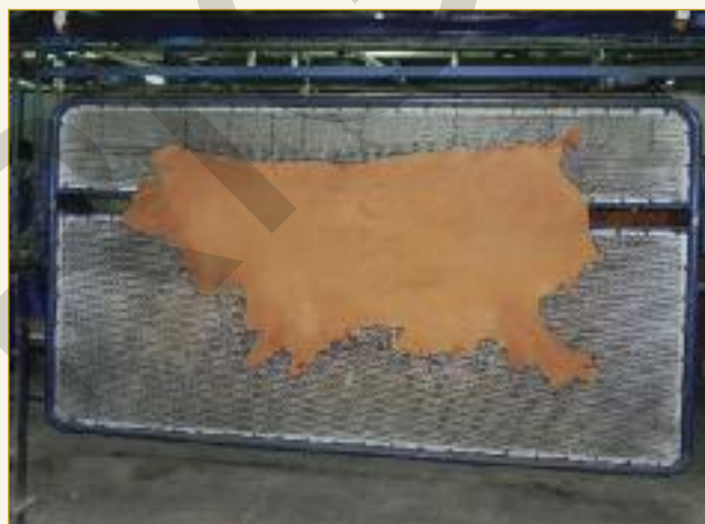
There are two toggle drying units, and a feature is the closeness of the placing of toggles around the sides to best maintain shape.
