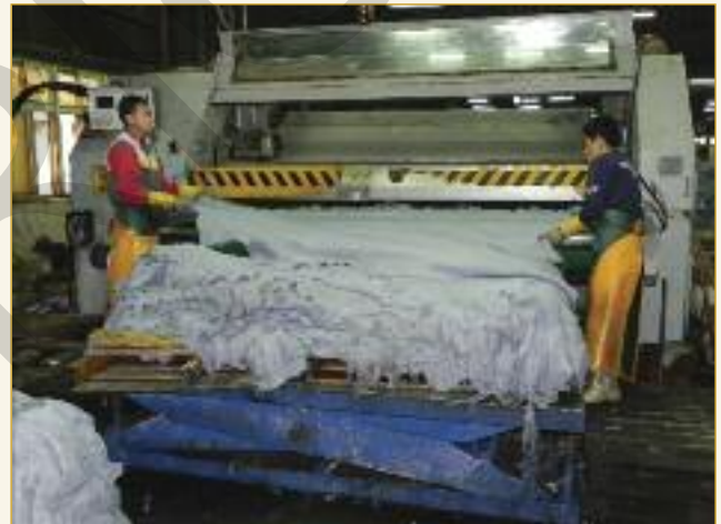
After sorting, the wet blue hides are samm/set. The hides are sided on a beam after blue splitting; the flesh splits remain as whole hide splits.
