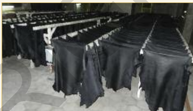
The interior of one of the suspension drying rooms. There is a second row of hanging rails set above those shown, and these are serviced from an elevated platform that runs on tracking so that it can be moved along the full length of the drying room.
