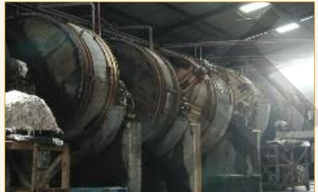
The tanning department comprises eight tanning drums. Four of these have been manufactured locally.
