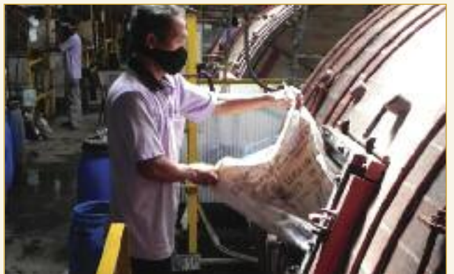
Both the dyeing and tanning drums are serviced from elevated platforms running along the rear of the drums.
