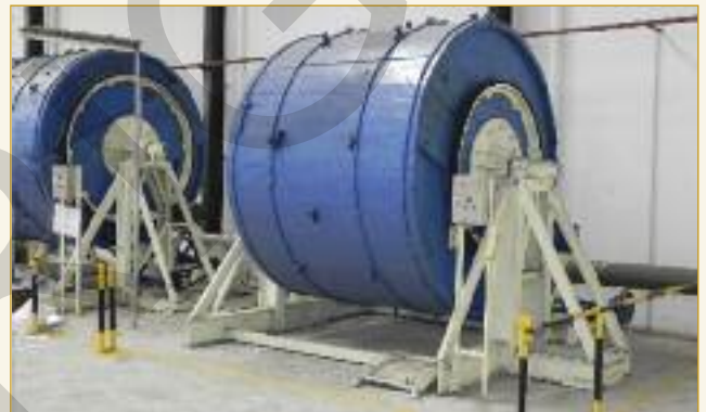
The two milling drums in the finishing department are made locally. They are mounted on a steel framework so that they can be readily repositioned.
