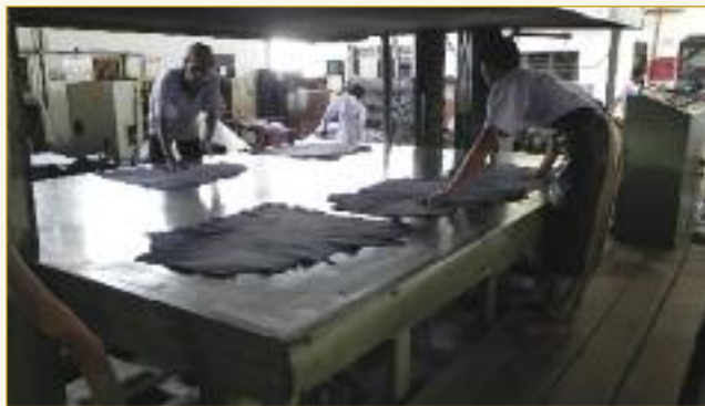
All of the sheep and goat skins manufactured for shoe upper leather are vacuum dried after samm/setting. This operation is then followed by softening using a feed-through staking machine.
