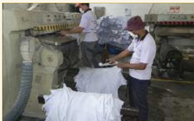
As each skin is shaved, it is checked for shaved substance.
