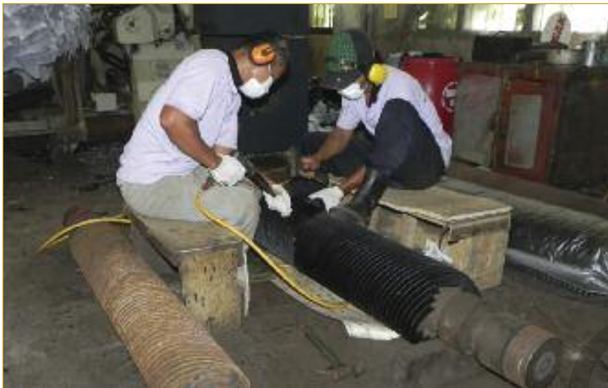
The tannery needs to be very self sufficient. In addition to plant and machinery of local manufacture, the maintenance department is comprehensive. The photograph shows shaving cylinders being rebladed.
