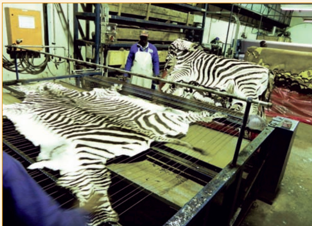
Zebra being wetted after sewing any flay cuts together, followed by drying while stapled to drying boards for flattening.
