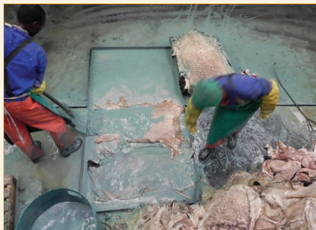
Painting with sulphide/lime paint for hair loosening
