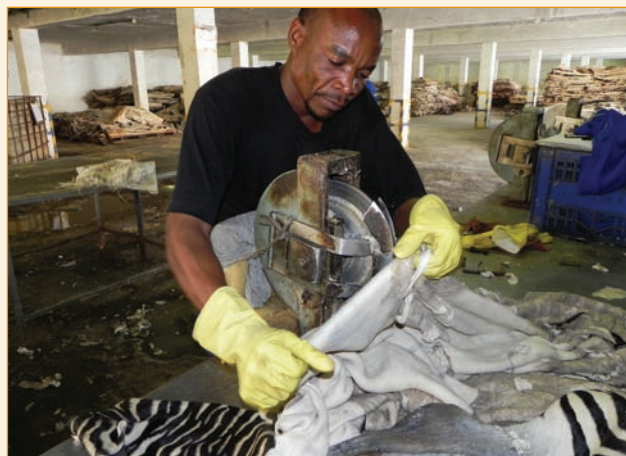
Wheel shaving zebra skins to remove surplus flesh and achieve uniformity of substance. This is a very skilled operation and cannot be replaced successfully by other methods.
