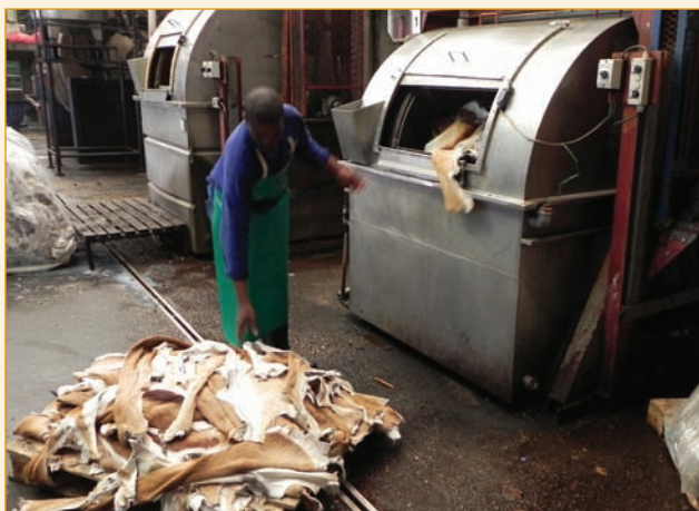
Springbok skins tend to form rolls in retanning/dyeing. To avoid this action the skins are stapled belly to belly before loading the tricompartmental processing vessel.
