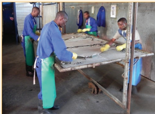
This toggling unit is dedicated to small skins, and drying is by forced air draft without any additional heat.
