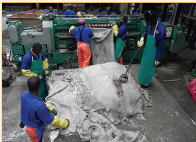
Metal detectors are used to scan each piece for buck-shot (oryx in this example) before lime splitting to avoid blade damage.
