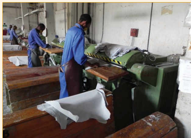
Buffing is a critical operation in the manufacture of suede leathers, and each goatskin is inspected for quality of the nap.
