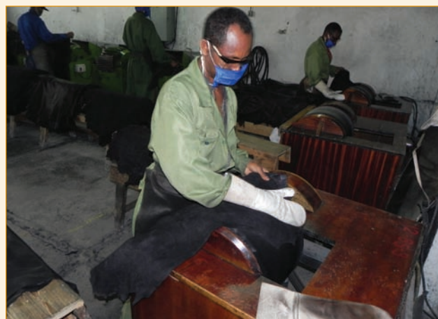
After wheel staking, the grain of the sheepskins are smoothed and flattened using a hand polishing wheel.
