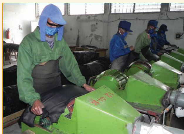
Wheel staking is applied after cylinder staking to further soften, but more selectively across the piece
