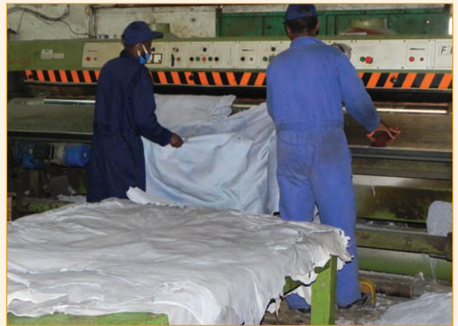
There are five shaving machines used within the bovine production plant. One for whole hides, and four for side leathers.
