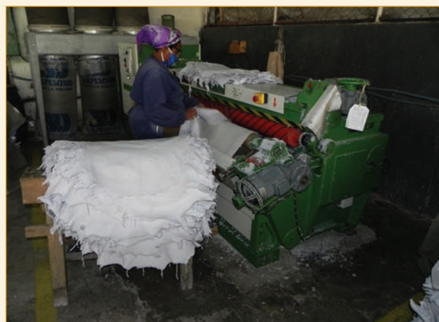
Sheepskins are first stretched and softened using a cylinder staking machine.
