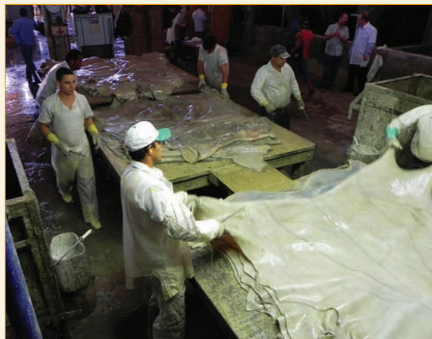
Lime fleshed goods are trimmed, inspected then loaded onto a flat top truck for transfer to the lime-splitting operation.
