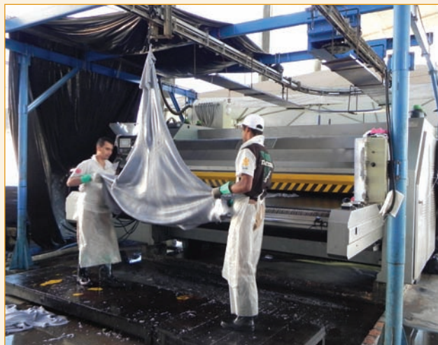
Tanned hides are received from the final delivery track by the operatives who open each hide for presentation to the samm/setting operation.
