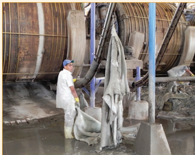
The limed hides are dumped into the area behind the liming drums, then hooked onto a delivery line feeding the lime fleshing operation.
