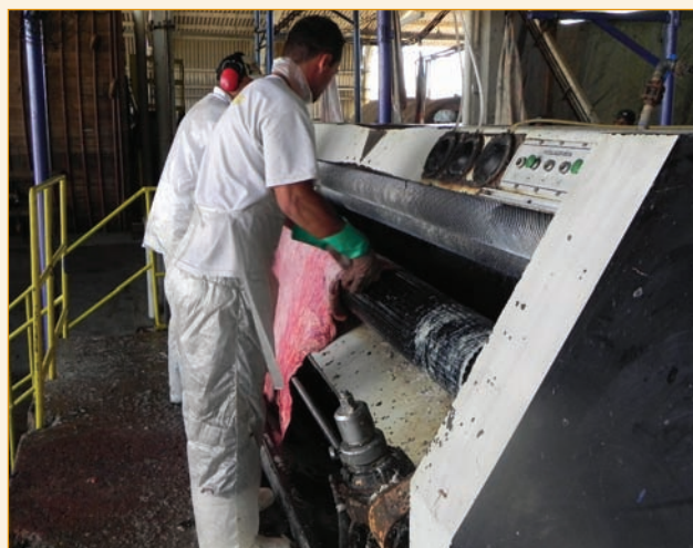
Fresh hides are often loaded onto the delivery track directly from the bed of the hide delivery truck. The feed is directly into the fleshing machine, with the fleshed hides dropping to the hide-stamping station.
