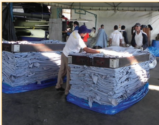
After grading, the hides are folded and loaded onto pallets. A box-template is used to ensure that the hides are uniformly stacked, before the loaded pallet is sealed and stored in the dispatch warehouse.
