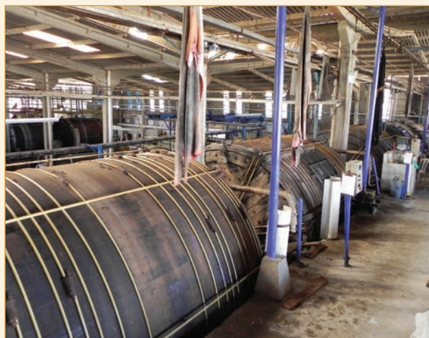
Once assessed for quality, then weighed on track, the hides are delivered to the designated drum according to individual weight.
