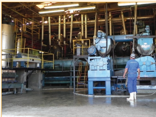
The rendering plant processes both green fleshings from the tannery, and bones delivered from the abattoirs. The recovered oils are filtered using a filter press, and then settled into various grades before storage and sale.
