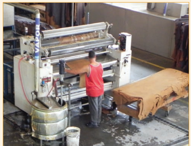
Combinations of waxes and oils at different levels of application are applied using roller coating machines.
