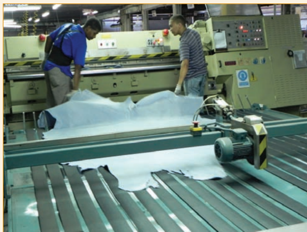
Grain splits are sided for shoe upper leathers after blue splitting. The cutting blade that is used for siding leathers is fitted into a stainless steel siding frame and thus avoids the use of hand knives.
