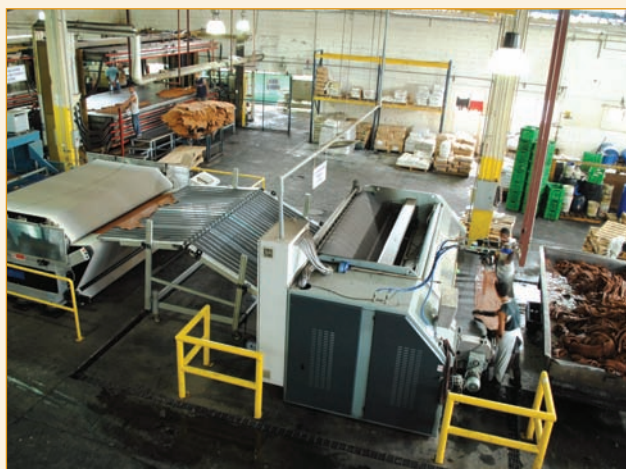
After dyeing/retan, the samm/setting of side leathers is followed by wet stretching/staking before vacuum drying.
