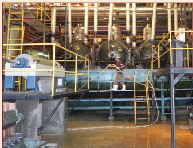
Fleshings and bones are first macerated, then heat rendered under pressure in the series of autoclaves.
