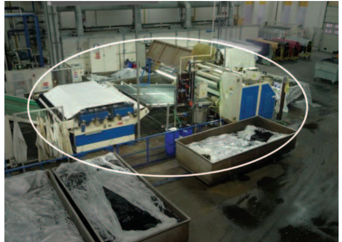
4. The "wet" stretching machine in line between samm/setting and vacuum dryer feeder
