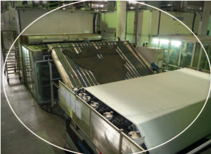
3. The "wet" stretching machine before TAIC.
