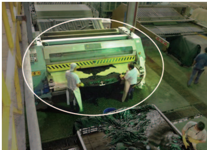
1. The through-feed samm/setting machine. Beginning of the just-in-time line.
