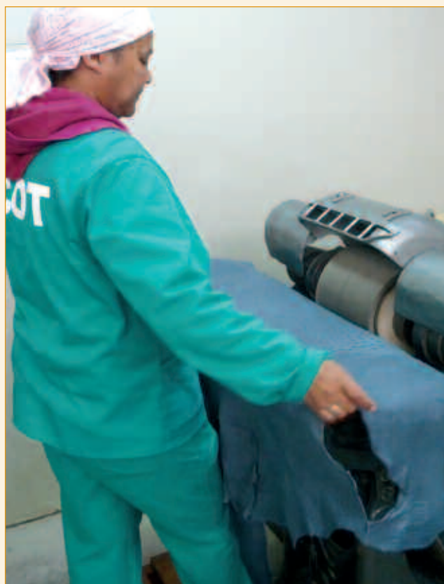
Polishing aniline finished leathers.
