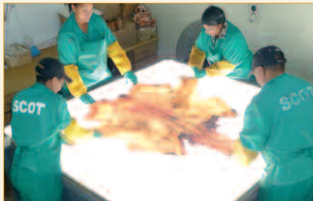
All skins are scanned after fleshing to measure area.
