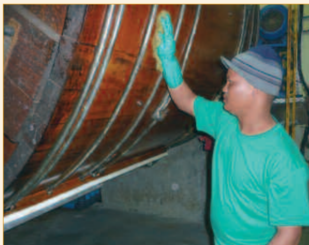
Considerable care is taken of the plant and machinery. Image shows the wooden drums being hand oiled.
